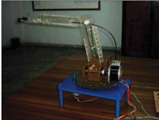
**Fig. 1:** Pick and Place Robot with Gripper Hand (Kabir *et al.*, 2003)
