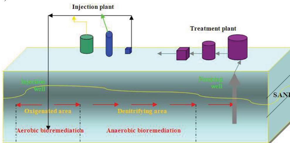
**Fig. 1:** Schematic in situ bioremediation
