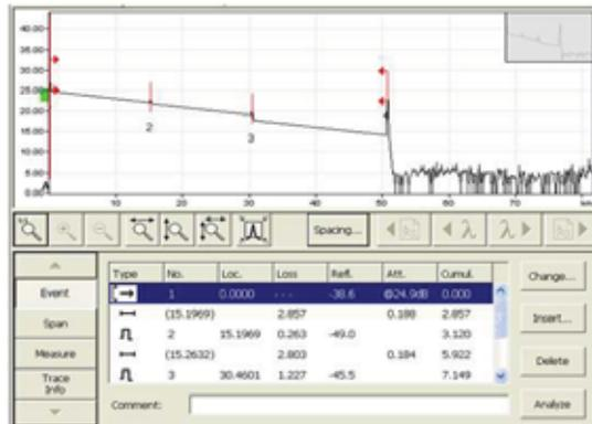
Fig. 9: The optical power level in line 2 are decreasing. Fig. 10: Execution display for line 2 in an emulation software.
