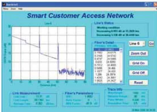
Fig. 17: The optical power level in line 1 are decreasing
