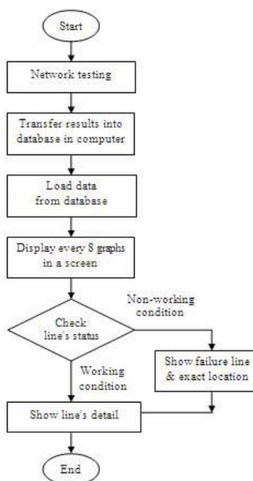
Fig. 1: Flow chart for mechanism of CFDS detection.
