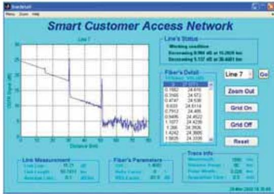
Fig. 19: The optical power level in line 7 are decreasing 0.984 dB at 15.2020 km and 5.137 dB at 30.4601 km.
