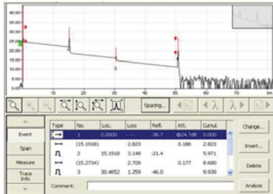
Fig. 11: The optical power level in line 3 are decreasing. Fig. 12: Execution display for line 3 in an emulation software.
