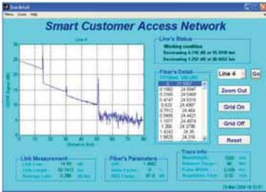
Fig. 13: The optical power level in line 4 are decreasing
