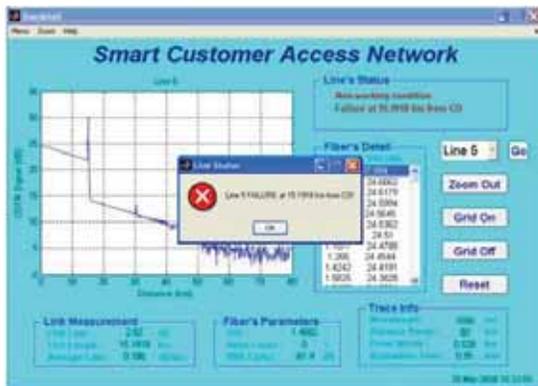
Fig. 15: Line 5 is failure at 15.1918 km when the attenuation at optical attenuator set as 5 dB.
