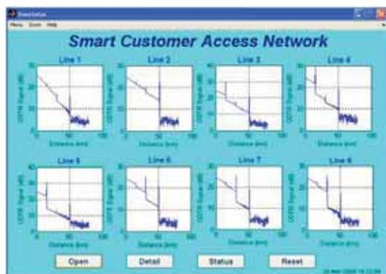
**Fig. 5:** Every 8 graphs display in Linestatus window for centralized monitoring.
