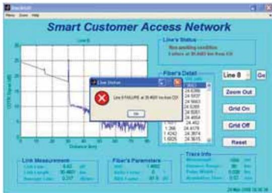
Fig. 21: Line 8 is failure at 30.4601 km when the attenuation at optical attenuator set as 5 dB.
