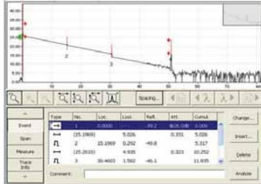
Fig. 7: The optical power level in line 1 are decreasing. Fig. 8: Execution display for line 1 in an emulation software.
