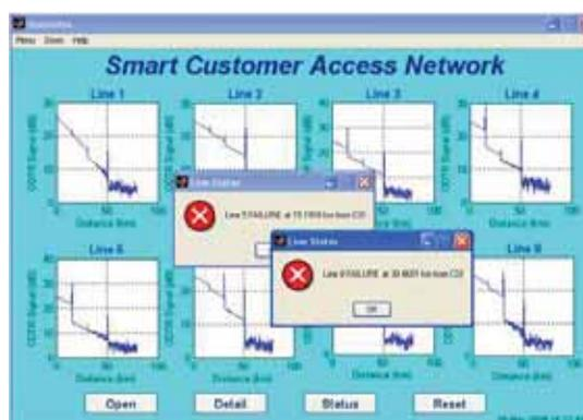
**Fig. 6:** Two failure messages display to show the failure locations in the optical network.
