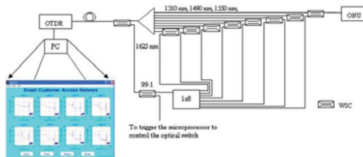
Fig. 2: The interconnection of optical switch to splitter and microprocessor system.
