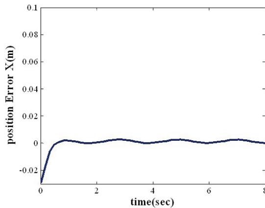
**Fig. 7:** Tracking error of  $X_d$  in the task space
