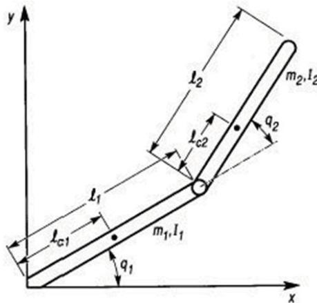
**Fig. 1:** Two-Link Elbow Robot Manipulator
