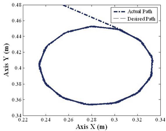
Fig. 4: Trajectory of end effector in the task space
