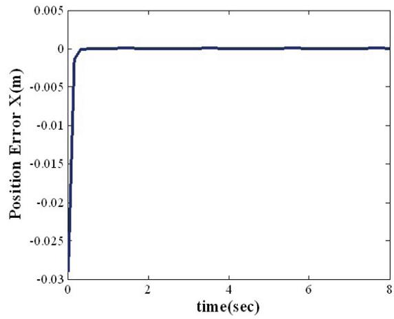
Fig. 2: Tracking error of  $X_d$  in the task space
