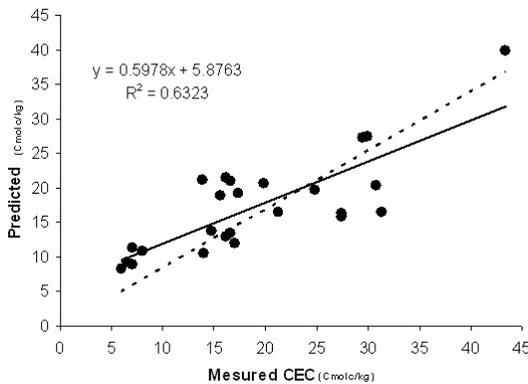
**Fig. 5:** The scatter plot of the measured versus predicted CEC
