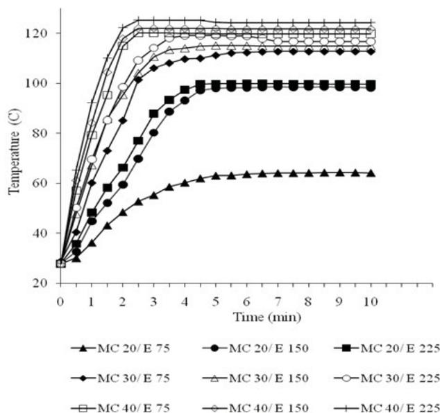
**Fig. 1:** The temperature changes of rice bran affected by different conditions of OMH (MC20/E75-MC40/E225 = Rice bran with moisture content of 20, 30 and 40% combined with electrical field strength of 75, 150 and 225 Vcm<sup>-1</sup>; Values are means of triplicate samples)
