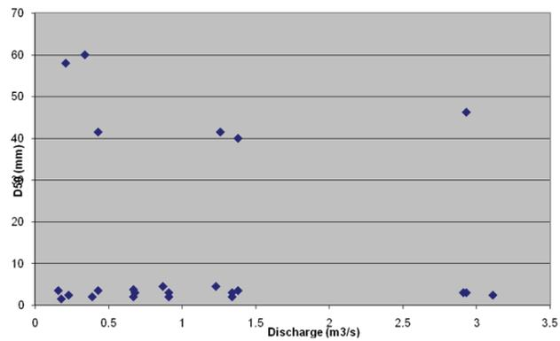
**Fig. 2:** Relation Between Values of  $D_{50}$  in mm and Average Discharge in  $m^3/s$  for Dengar, Mengkibol and Madek River in Johor
