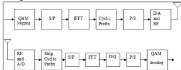
**Fig. 3:** An OFDM Modulator/Demodulator
