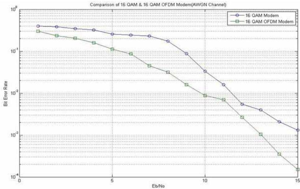
Fig. 5: Comparisons of 16 QAM & 16 QAM OFDM Modem (AWGN)
