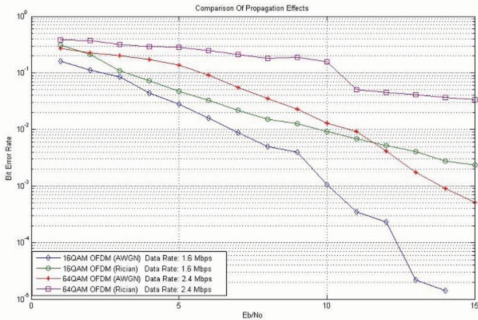
Fig. 7: Comparison of Propagation Effects
