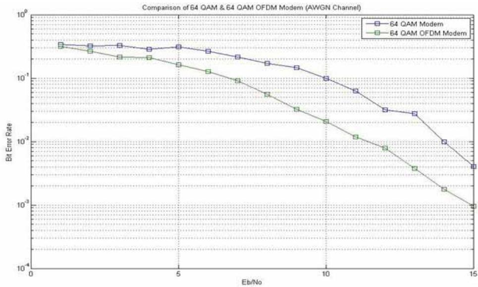
Fig. 6: Comparisons of 64 QAM & 64 QAM OFDM Modem (AWGN)
