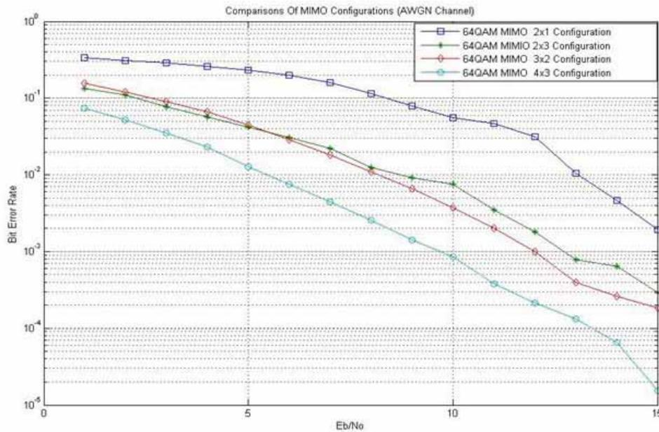
Fig. 8: Impacts of MIMO Configurations
