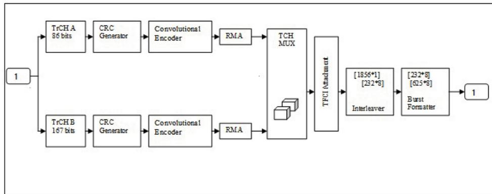
**Fig. 2:** Evolved EDGE Flexible Layer One (FLO) Architecture
