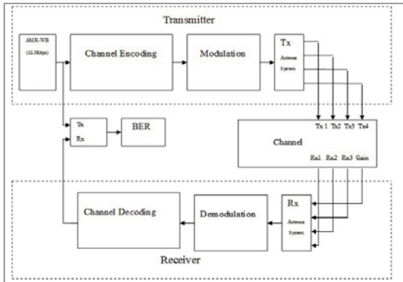
**Fig. 1:** Evolved EDGE Transceiver Block Diagram
