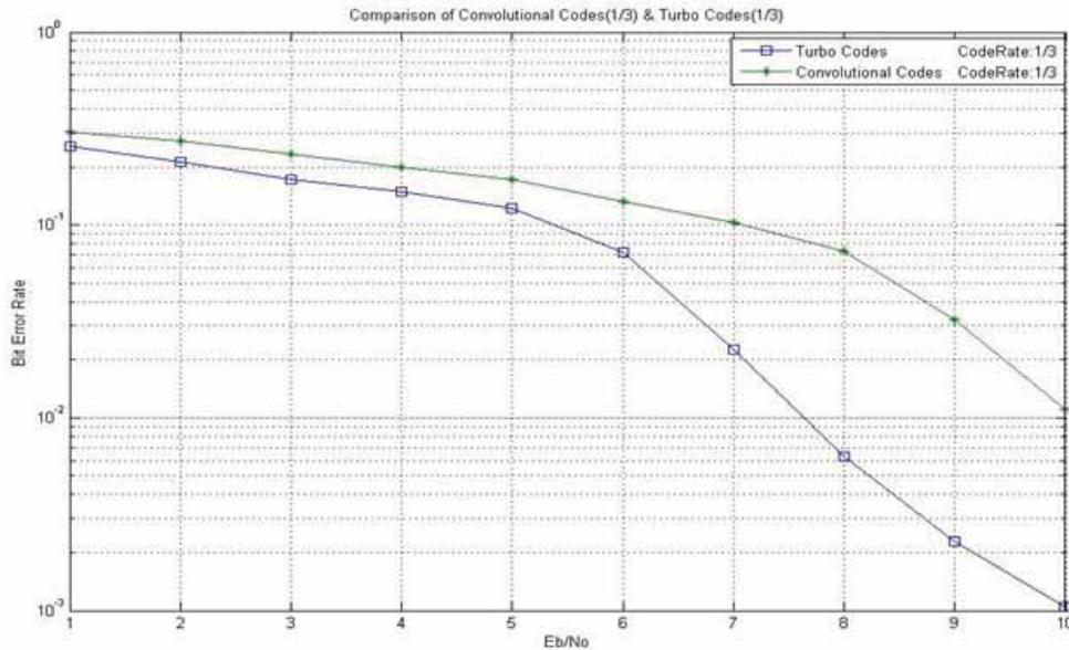
**Fig. 9:** Comparison of Convolutional Code (Rate: 1/3) and Turbo Code (Rate: 1/3)
