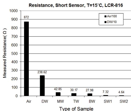
Fig. 5: Resistance measurements for the air and different water liquids for the short probe.
