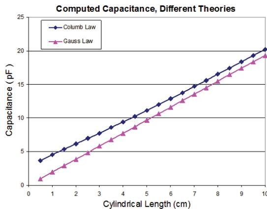
**Fig. 10:** Computed air capacitance values from two theories.
