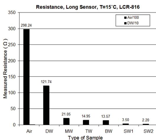
Fig. 6: Resistance measurements for the air and different water liquids for the long probe.
