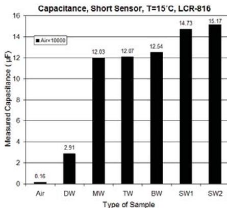
**Fig. 3:** Capacitance measurements for the air and different water liquids for the short probe.
