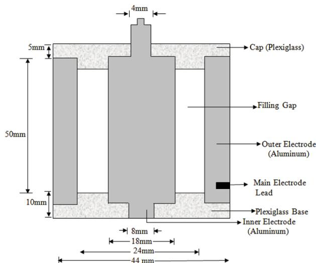
**Fig. 1:** Design of the cylindrical capacitive cell probe.
