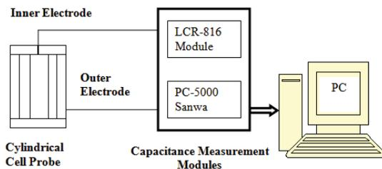
**Fig. 2:** Block diagram of the experiment for capacitance measurements.
