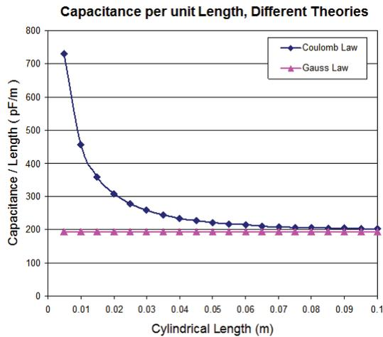
**Fig. 9:** Computed air capacitance per unit length from two theories.
