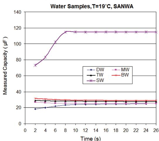
**Fig. 11:** Time variation of the measured capacitance for the water samples.
