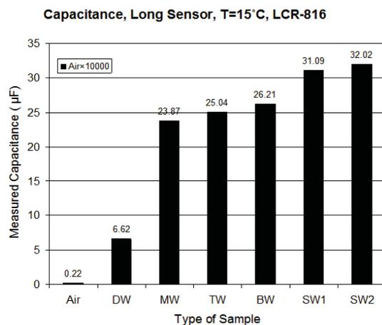
**Fig. 4:** Capacitance measurements for the air and different water liquids for the long probe.
