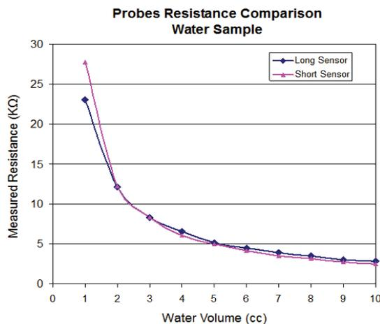
**Fig. 8:** Resistance variation for different volumes distilled water liquid filling.
