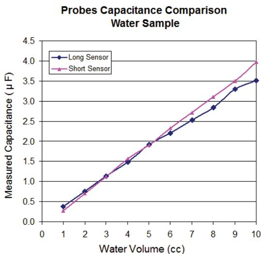
**Fig. 7:** Capacitance variation for different volumes distilled water liquid filling.
