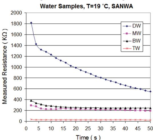
**Fig. 12:** Time variation of the measured resistances for different water samples using DMM module.
