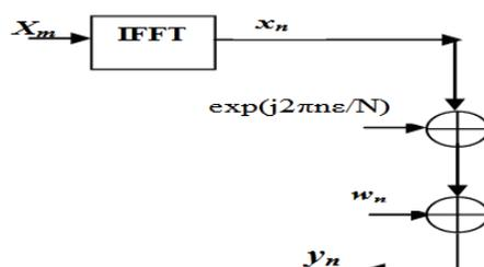
Fig. 2: Frequency offset model
