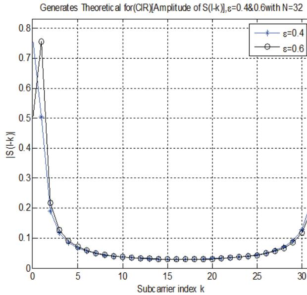
**Fig. 3:** ICI Coefficients (Amplitude ) for N=32 carriers
