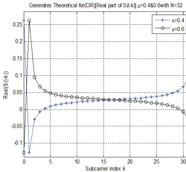
**Fig. 4:** ICI Coefficients (Real part) for N=32 carriers
