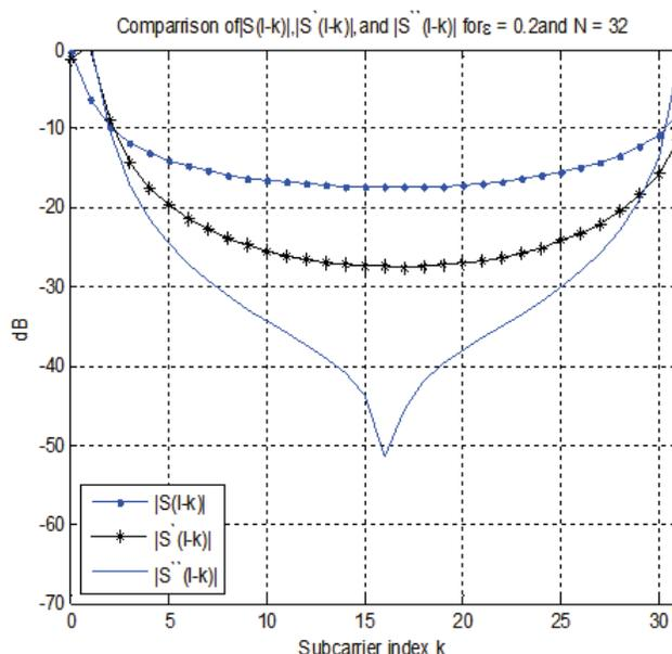
**Fig. 6:** Comparison of  $|S(l-k)|$ ,  $|S'(l-k)|$ , and  $|S''(l-k)|$  for  $N = 32$  and  $\epsilon = 0.2$
