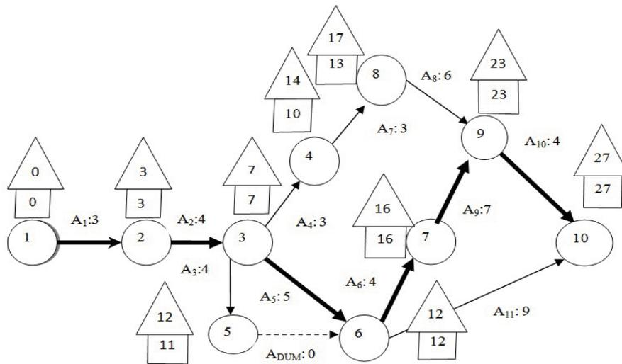
**Fig. 1:** Critical path, earliest start and finish, latest start and finish in normal conditions
