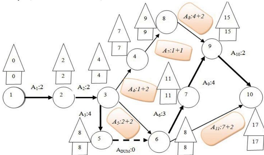
**Fig. 2:** Critical path, earliest start and finish, latest start and finish and mechanism of stretching noncritical activities
