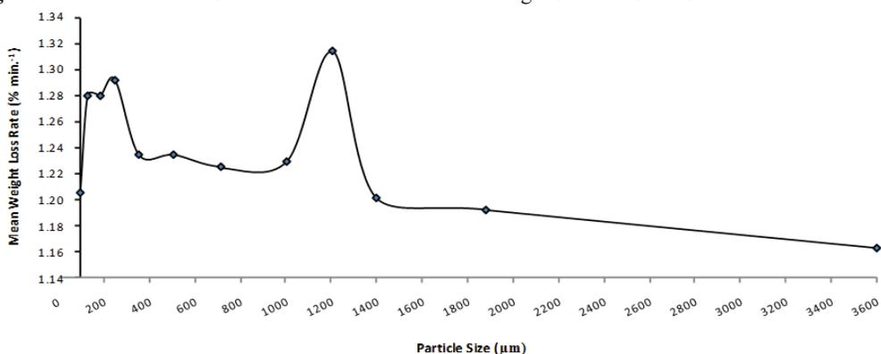
Fig. 4: Effect of Particle Size on Weight loss characteristics of Moringa Oleifera Seed Shell at high temperature
