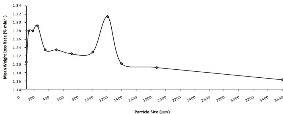
Fig. 3: Effect of Particle Size on Volatile Matter of Moringa Oleifera Seed Shell.
