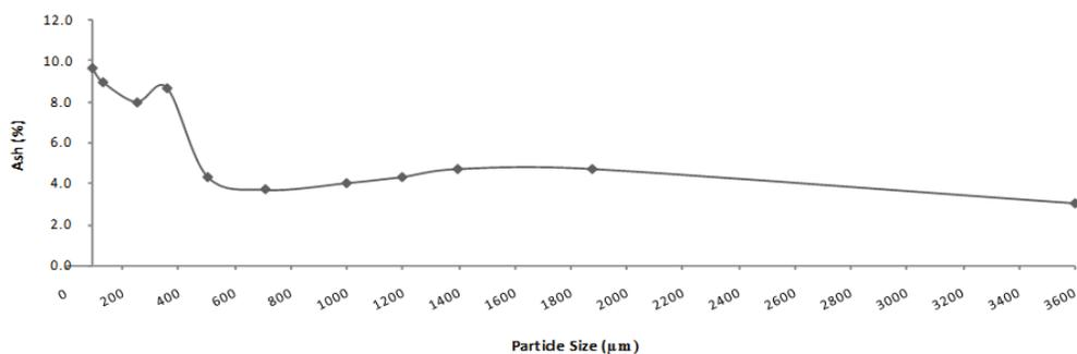
Fig. 5: Effect of Particle Size on Ash content of Moringa Oleifera Seed Shell
