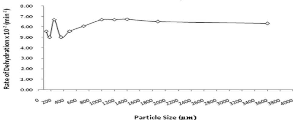
Fig. 2: Effect of Particle Size on Rate of Dehydration of Moringa Oleifera Seed Shell
