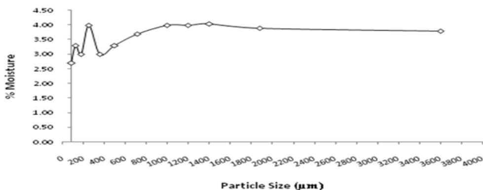
Fig. 1: Effect of Particle Size on Moisture Content of Moringa Oleifera Seed Shell
