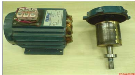
Fig. 11: Complete copper rotor of induction motor
