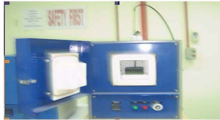
Fig. 5: Furnace chamber (Where copper is melted in rotor slots)
