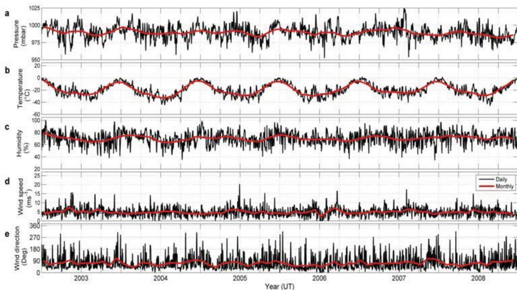
**Fig. 2:** Temporal variations of daily-mean surface meteorological measurement for the period from 2003 to 2008 at Scott Base station, Antarctica. Note that the red solid lines show for monthly-mean values, and the year marks on the figure denotes the middle of the year
