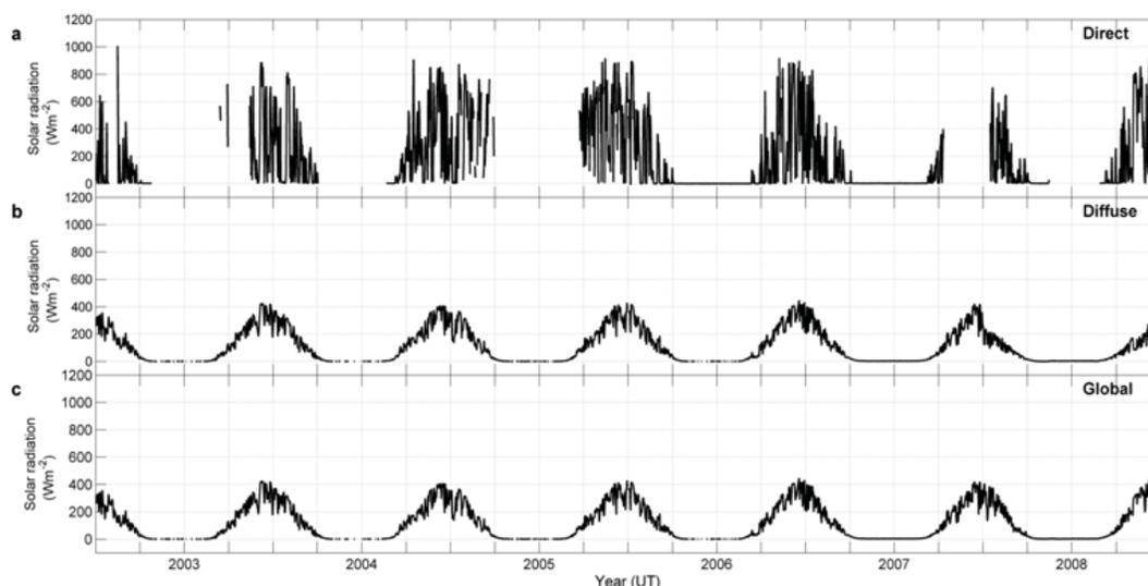
**Fig. 4:** Temporal variations of solar radiation for direct, diffuse and global measurements during the period of 2003 to 2008 at Scott Base station, Antarctica
