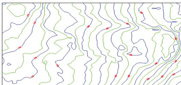
Fig. 9: Contour Map of terrain of site no.8 (Contour interval =1m)
