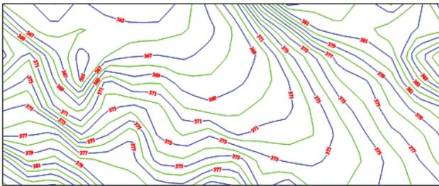
**Fig. 4:** Contour Map of terrain of site no.3 (Contour interval =1m)
