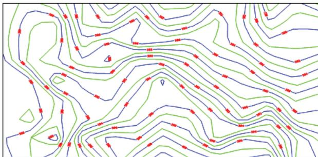
**Fig. 3:** Contour Map of terrain of site no.2 (Contour interval =1m)
