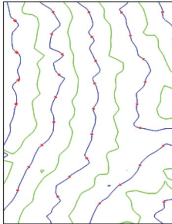
**Fig. 6:** Contour Map of terrain of site no.5 (Contour interval =1m)
