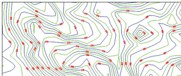
**Fig. 5:** Contour Map of terrain of site no.4 (Contour interval =1m)
