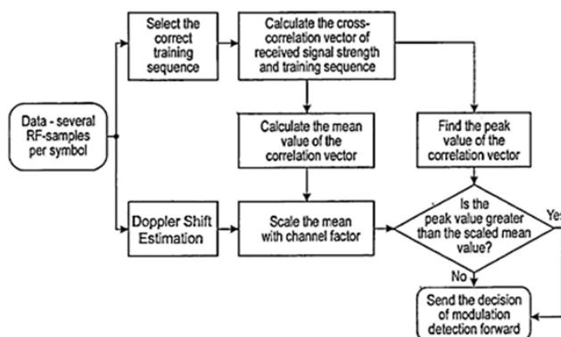
Fig. 4: Modulation detection algorithm
