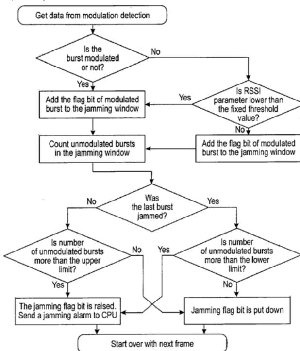
Appendix: Fig. 8: The jamming Detection Algorithm in details (Kurahila, M., M. Torvinen, 2006)
