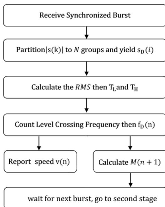
**Fig. 2:** Signal Flow of the Proposed Algorithm.
