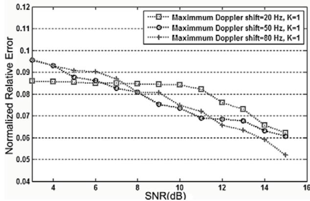
Fig. 5: Normalized relative error in various Doppler shifts.
