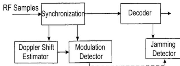
**Fig. 3:** The overall procedure of jamming detection algorithm
