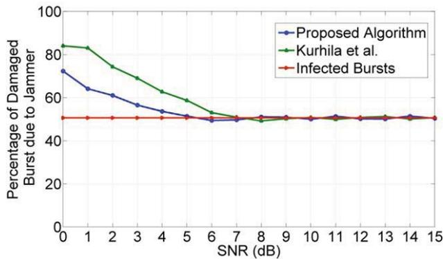
Fig. 7: Percentage of corrupted bursts due to jammer, the constant curve is expected corruption percentage and the other curves are the algorithms' estimation. SJR=8 dB, Lower Limit=9, Upper Limit=12, Doppler Shift=20 Hz. RSSI=-60dBm.
