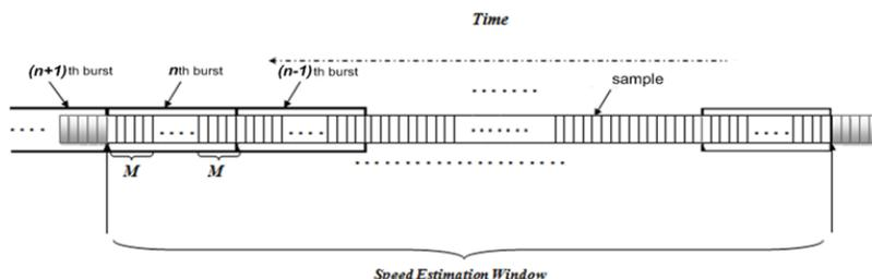
**Fig. 1:** The structure of speed estimation window.
