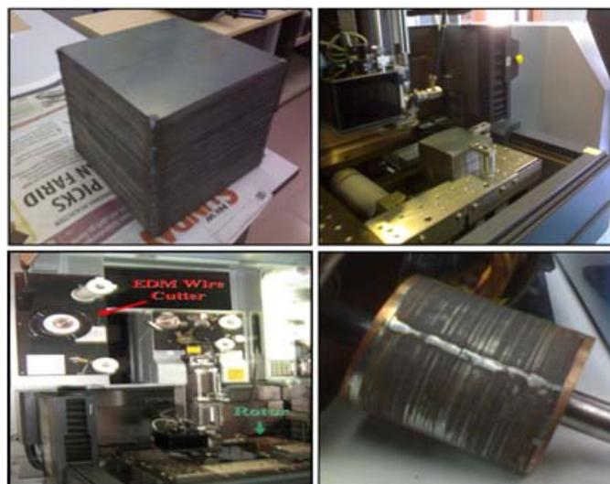
**Fig. 2:** Copper Rotor Fabrication Procedures.
