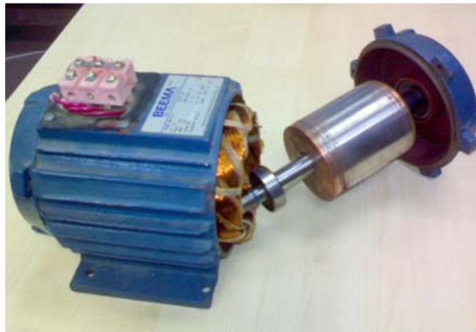
**Fig. 4:** Copper Rotor assemble into the Induction Motor Stator.
