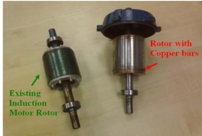
**Fig. 3:** Copper Rotor of Induction Motor after Milling Process.
