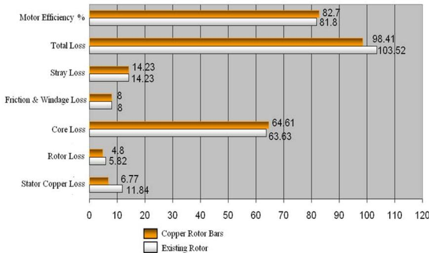
**Fig. 5:** Copper Rotor and Existing Rotor Performance.
