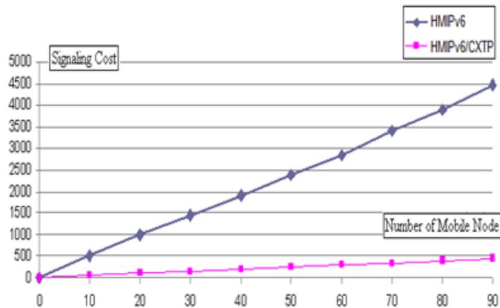
Fig. 6: Signaling Cost versus Number of Mobile Node
