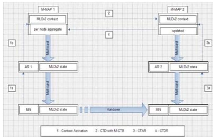
Fig. 4: MN handover flow in M-HMIPv6 with CXTP.
