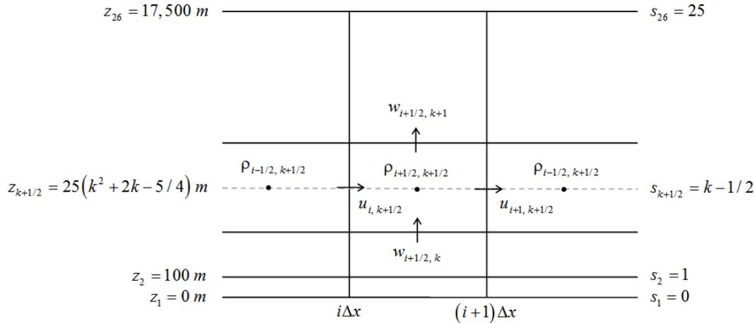
**Fig. 1:** The grid of the simple model with the stretched grid.
