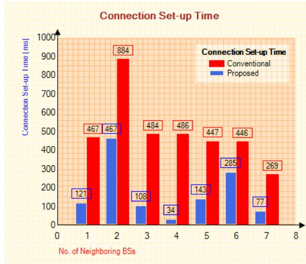
Fig. 15: Conventional vs. Proposed Connection Set-up Time
