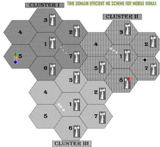
Fig. 4: Cell topology for simulation
