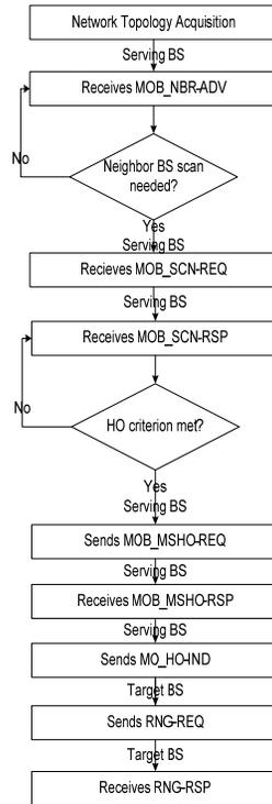
Fig. 7: Proposed HO Process message exchange
