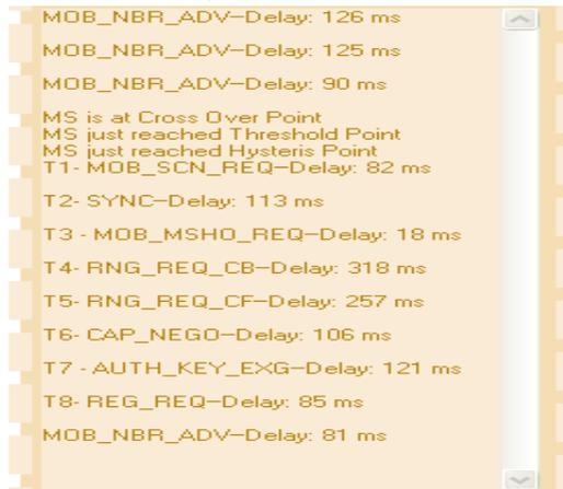
**Fig. 11:** MS HO results from Cell 5 to Cell 7 mobility model
