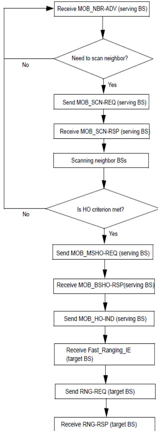
**Fig. 5:** Initiation of HO Process by MS (IEEE Standard for Local and Metropolitan Area Networks).
