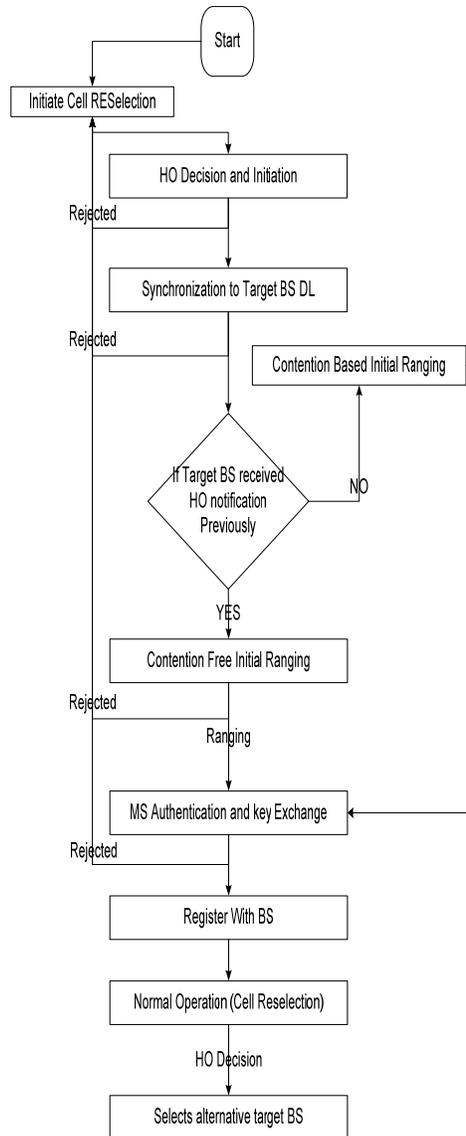
**FIG. 6:** SIMPLIFIED PROPOSED HO PROCESS
