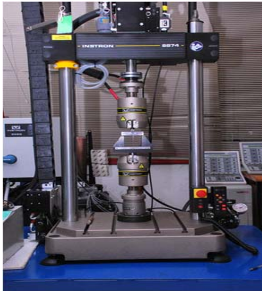
Fig. 3: The experiment setup of the INSTRON machine model 8874.
