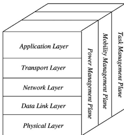
**Fig. 3:** The sensor networks protocol stack.
