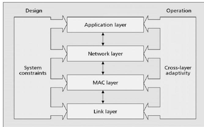
**Fig. 4:** Adaptive cross-layer design and operation.
