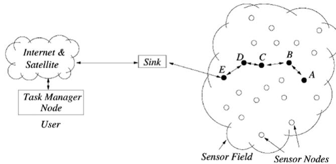
**Fig. 2:** connection architecture of wireless sensor networks.
