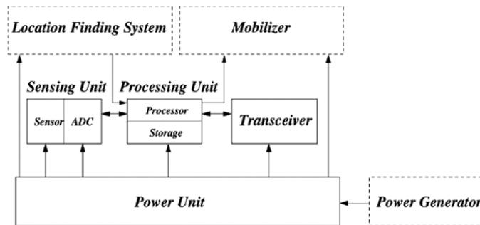
**Fig. 1:** The components of a sensor nodes.
