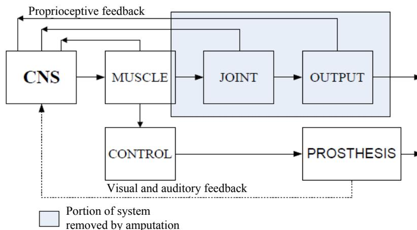
**Fig. 1:** Block diagram presenting relationship between normal and electromyographic control system (shaded area is removed by amputation) (Parker *et al.*, 2006)
