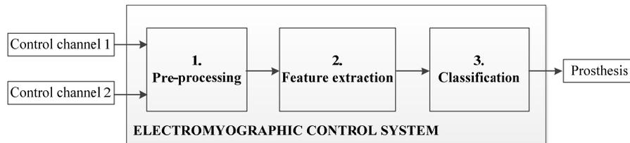
**Fig. 3:** The block diagram of an electromyographic control system (ECS) based on pattern recognition
