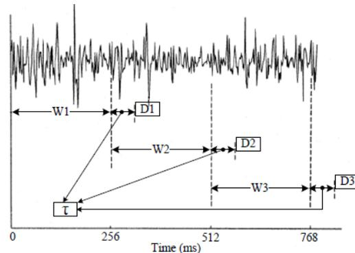
**Fig. 4:** Adjacent windowing technique. W: Window, D: Delay,  $\tau$ : time delay [Englehart & Hudgins, 2003]
