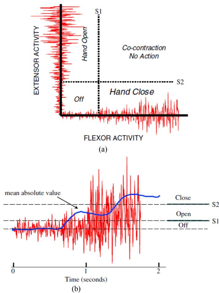
**Fig. 2:** (a) Two channels amplitude coded; (b) One channel amplitude coded myoelectric control (Parker *et al.*, 2006)
