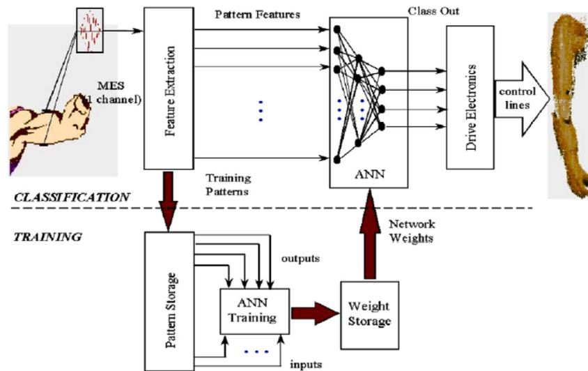
**Fig. 5:** Electromyographic control system using ANN as the classifier (Parker *et al.*, 2006)
