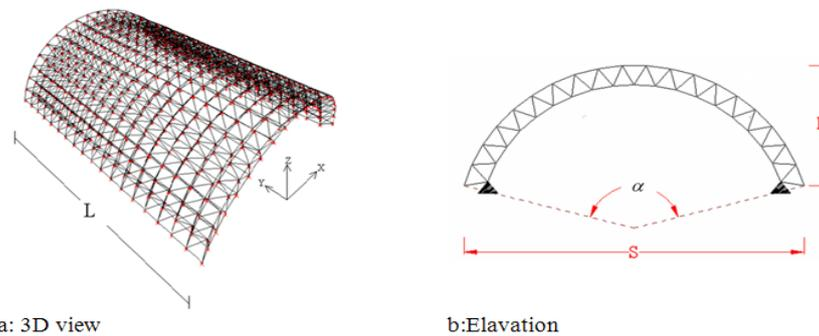
**Fig. 2:** General geometrical properties of models.
