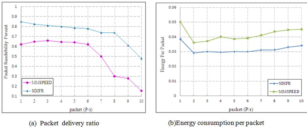
**Fig. 7:** (a) packets delivery ratio- (b) Energy consumption per packet.
