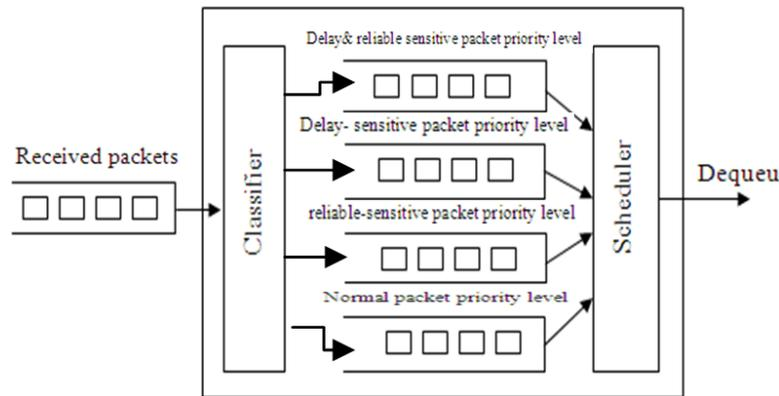
Fig. 5: Four-level M/G/1 queuing model.
