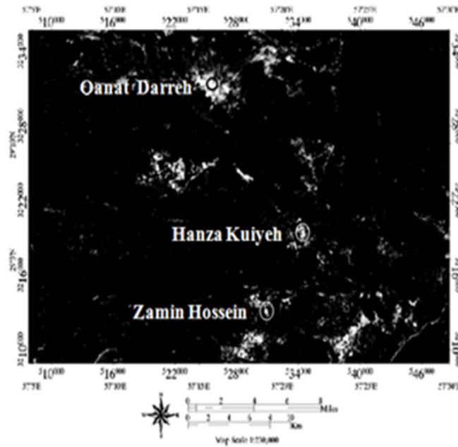
**Fig. 3:** The phyllic image that is prepared based on the eigenvector loadings (PC3) of table 2.
