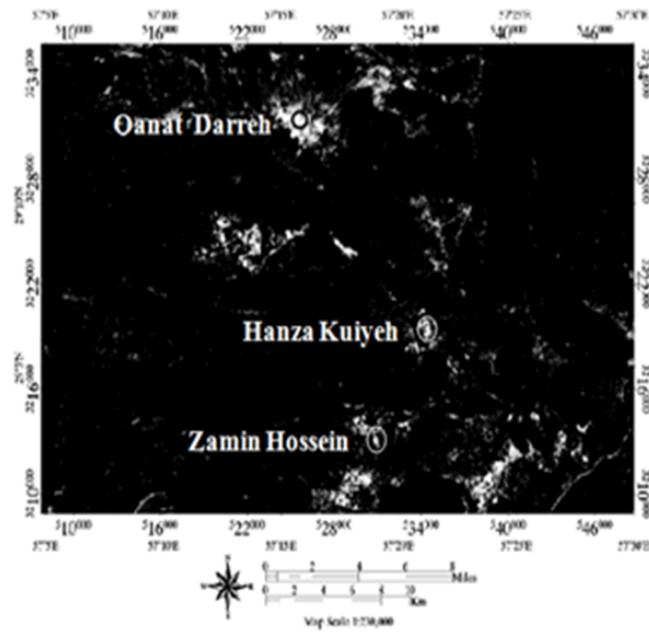
**Fig. 4.** The argillic image that is prepared based on the eigenvector loadings (PC3) of table 3.
