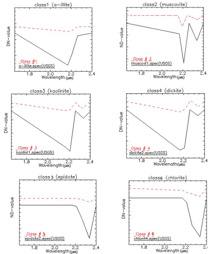
**Fig. 6:** Matching class spectra to USGS mineral spectral library.
