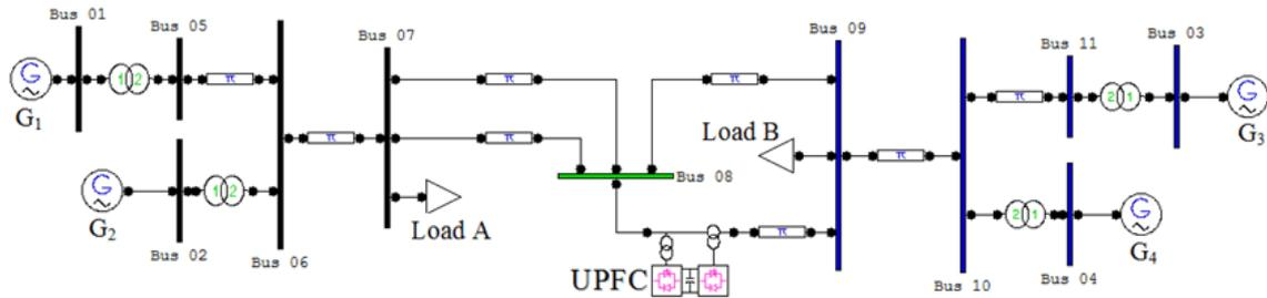
**Fig. 1:** Four-machine eleven-bus power system.
