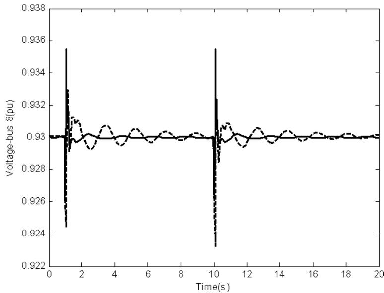
**Fig. 8:** Voltage of bus number 8 under scenario 2 in nominal load condition Solid (with UPFC); Dashed (without UPFC).
