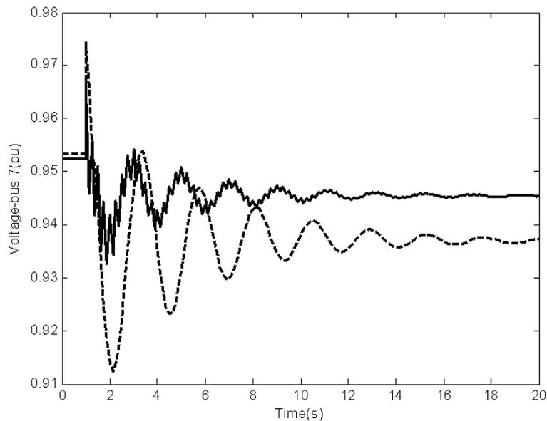
**Fig. 5:** Voltage of bus number 7 under scenario 1 in nominal load condition Solid (with UPFC); Dashed (without UPFC).
