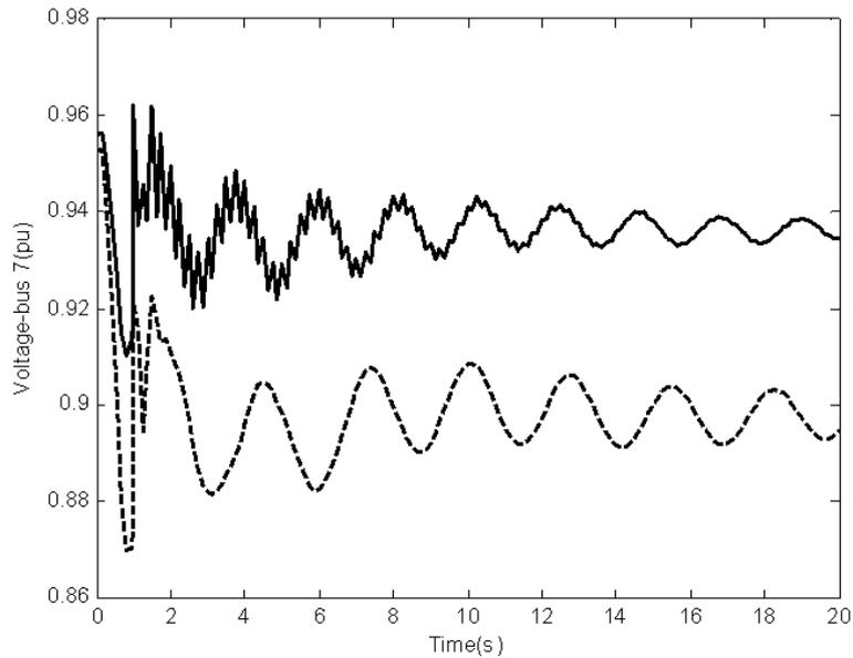
**Fig. 7:** Voltage of bus number 7 under scenario 1 in heavy load condition Solid (with UPFC); Dashed (without UPFC).
