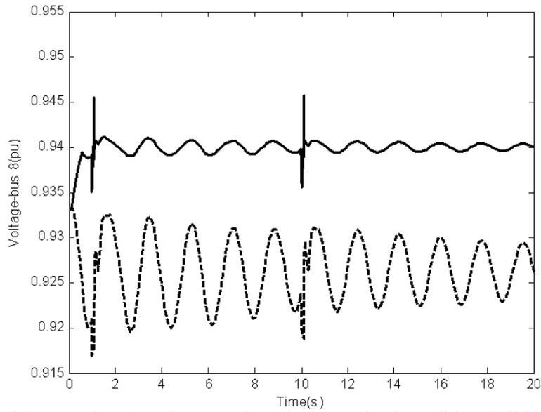
**Fig. 10:** Voltage of bus number 8 under scenario 2 in heavy load condition Solid (with UPFC); Dashed (without UPFC).
