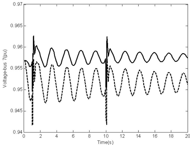
**Fig. 11:** Voltage of bus number 7 under scenario 2 in heavy load condition Solid (with UPFC); Dashed (without UPFC).
