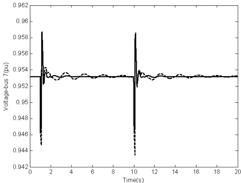
**Fig. 9:** Voltage of bus number 7 under scenario 2 in nominal load condition Solid (with UPFC); Dashed (without UPFC).
