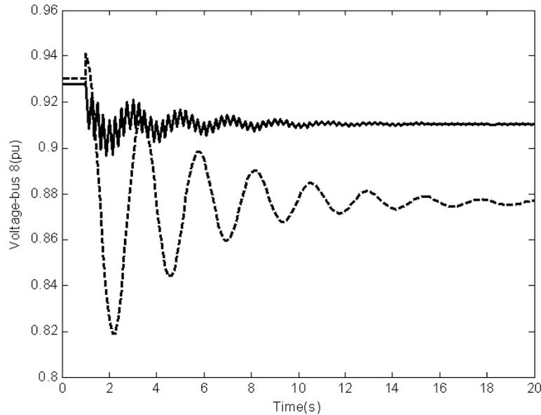
**Fig. 4:** Voltage of bus number 8 under scenario 1 in nominal load condition Solid (with UPFC); Dashed (without UPFC).
