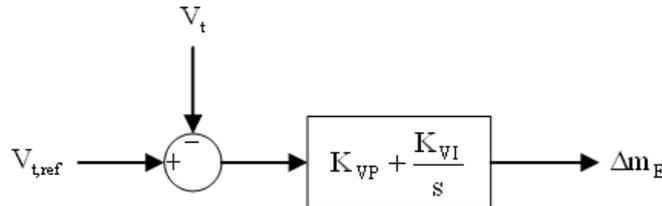
**Fig. 3:** Bus voltage controller.
