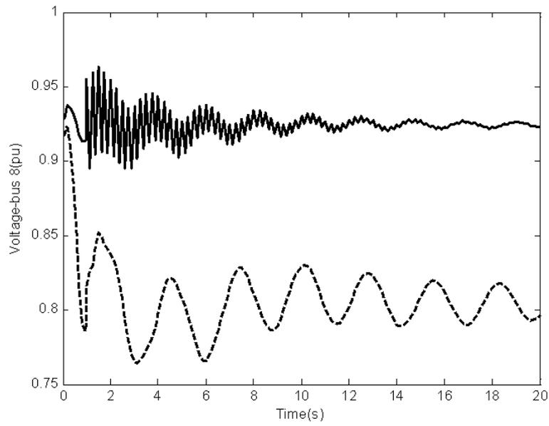
**Fig. 6:** Voltage of bus number 8 under scenario 1 in heavy load condition Solid (with UPFC); Dashed (without UPFC).
