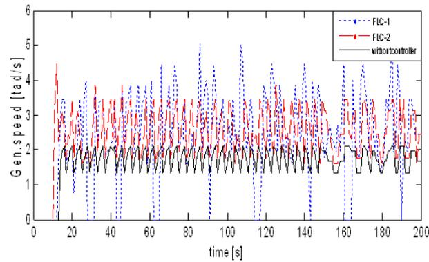
**Fig. 7.d:** Generator speed of wind turbine for pitch angle fixed and control in variatif wind speed
