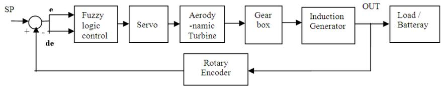
Fig. 2: Block diagram wind turbine with generator system
