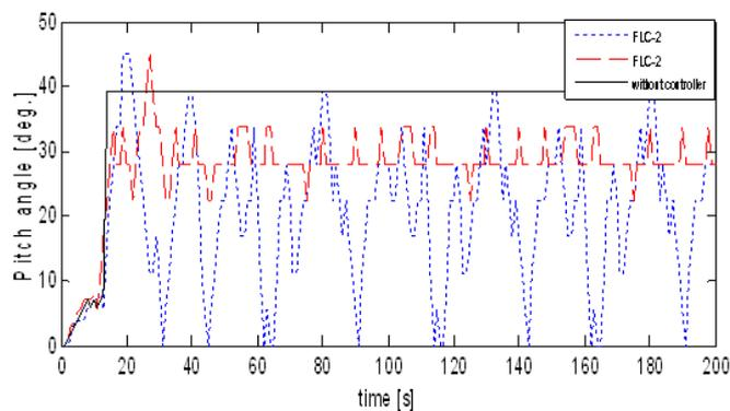
**Fig. 7.c:** Corresponding to change in wind speed from 4 to 7 m/s for three different variabel speed controllers.
