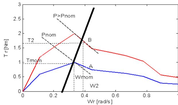
**Fig. 8:** Fixed-speed power regulator on the torque –speed plane
