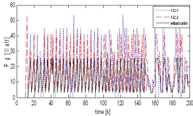
**Fig. 7.b:** Wind power generation at pitch angle fixed and control in wind speed variatif
