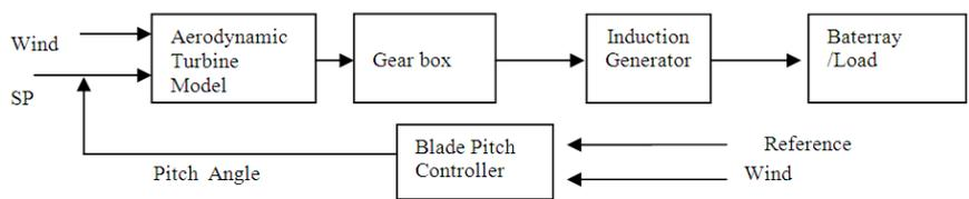
Fig. 1: A WECS block diagram with the capability to change the pitch angle
