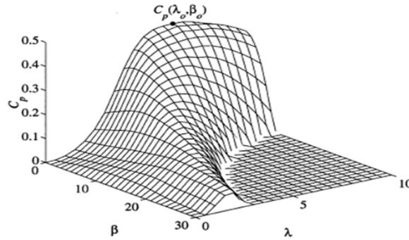
Fig. 3: Typical power coefficient  $C_p(\lambda, \beta)$ .
