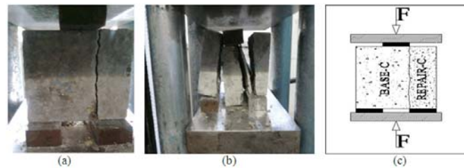
Fig. 5. the loading condition and mode of fracture: a. loading, b. two-layer mode fracture, c. single-layer mode of fracture
