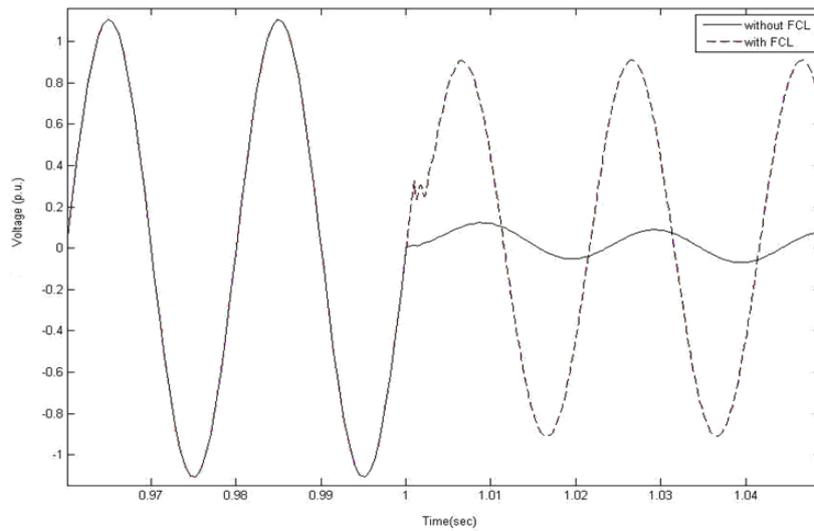
Fig. 4: the three-phase fault current with and without limitation strategy
