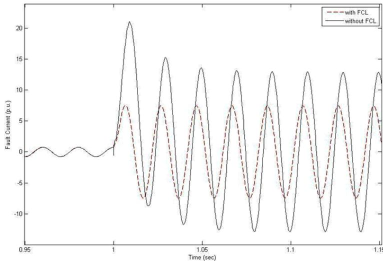
**Fig. 3:** the three-phase fault current with and without limitation strategy
