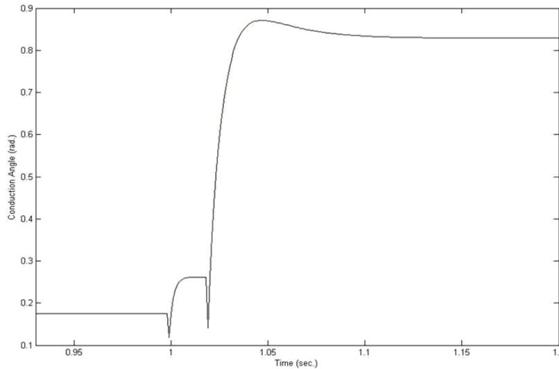
Fig. 5: the TCSC conduction angle
