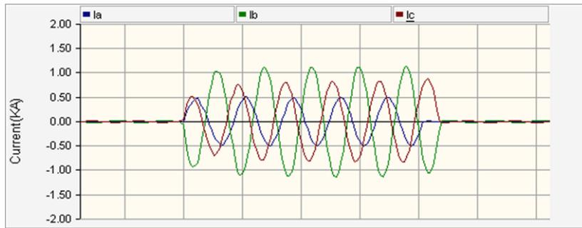
Fig. 2(c): Fault current waveforms with DG installation and using FCL
