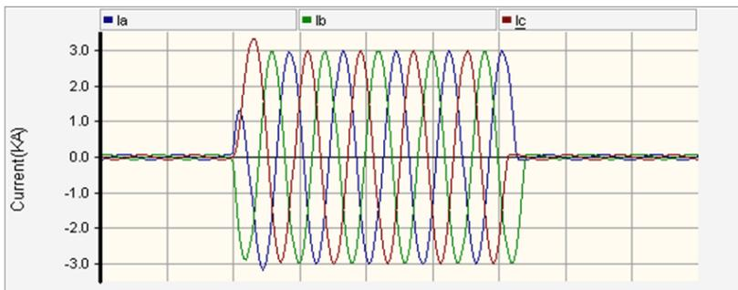
Fig. 3(b): Fault current waveforms with DG installation at P4 (fault at F2)
