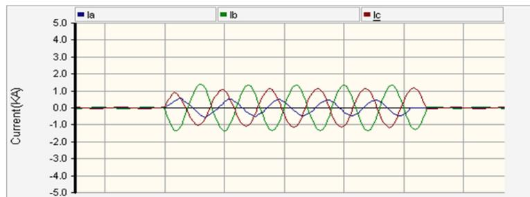
**Fig. 4(c):** Entire fault current waveforms with DG installation at P3 and using FCL (fault at F4)
