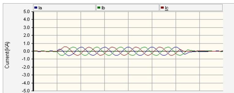
**Fig. 4(d):** fault current waveforms passes through recloser with DG installation at P3 and using FCL (fault at F4)
