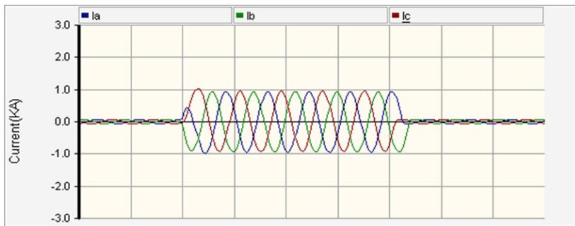
Fig. 3(a): Fault current waveforms without DG installation (fault at F2)
