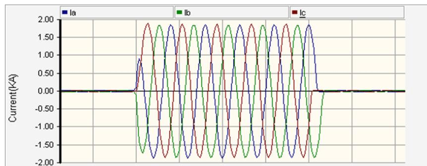
**Fig. 2(b):** Fault current waveforms with DG installation
