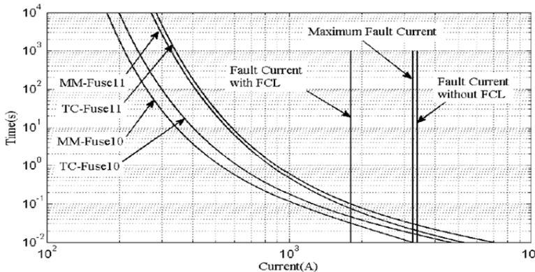
**Fig. 5(c):** MMT and MCT curves of fuse10 and 11
