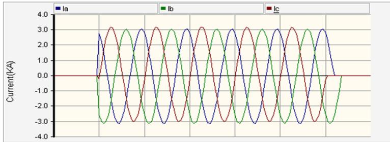
**Fig. 5(a):** fault current waveforms passes through fuse10 with DG installation at P1 (fault at F1)
