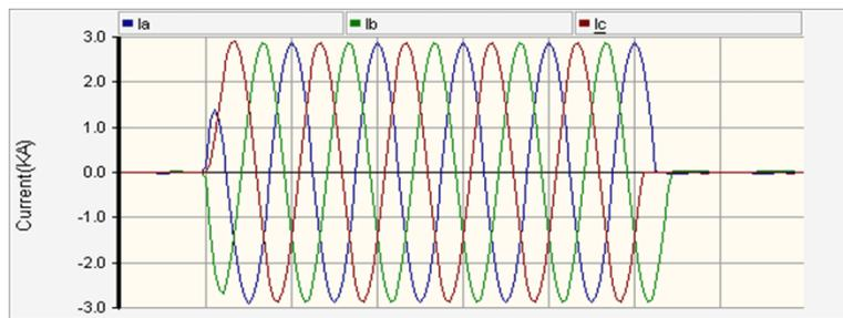
**Fig. 6(a):** fault current waveforms passes through fuse11 with DG installation at P2 (fault at F5)
