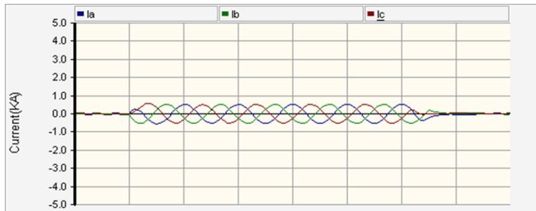
**Fig. 4(b):** fault current waveforms passes through recloser with DG installation at P3 (fault at F4)
