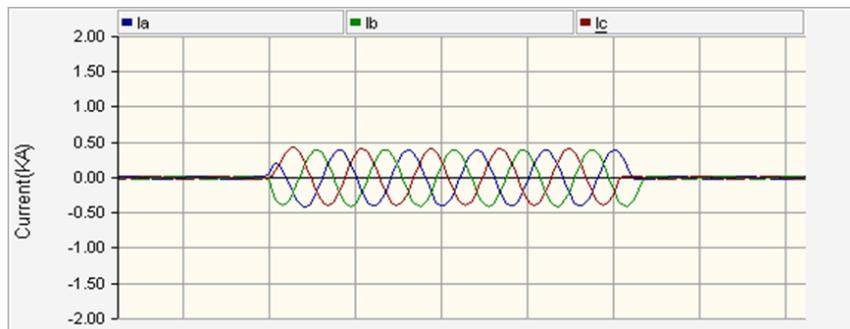
**Fig. 2(a):** Fault current waveforms without DG
