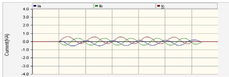
**Fig. 5(b):** fault current waveforms passes through fuse10 with DG installation at P1 and using FCL (fault at F1)
