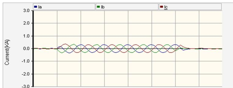
**Fig. 6(b):** fault current waveforms passes through recloser with DG installation at P2 (fault at F5)
