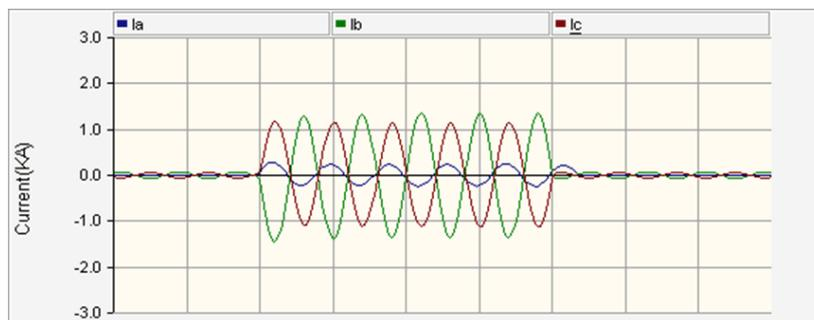
Fig. 3(c): Fault current waveforms with DG installation at P4 (fault at F2) and using FCL
