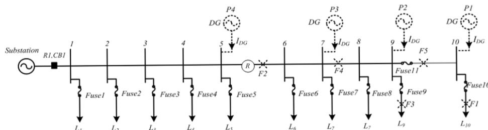
**Fig. 1:** Radial test system with DG and local loads
