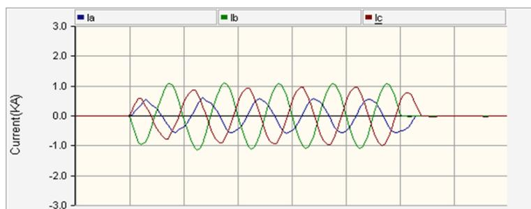
**Fig. 6(c)** fault current waveforms passes through fuse11 with DG installation at P1 and by using FCL (fault at F1)
