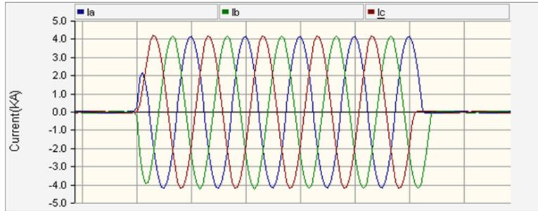
**Fig. 4(a):** Entire fault current waveforms with DG installation at P3 (fault at F4)
