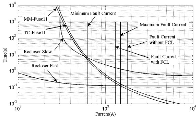
**Fig. 6(d):** coordination characteristics between recloser and fuse11
