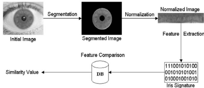
**Fig. 2:** steps of identification using biometric iris (“<http://www.iris-recognition.org>”).
