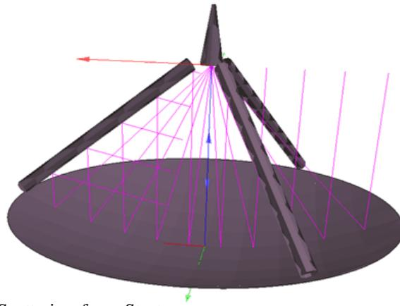
**Fig. 1.3:** Blockage and Scattering from Struts
