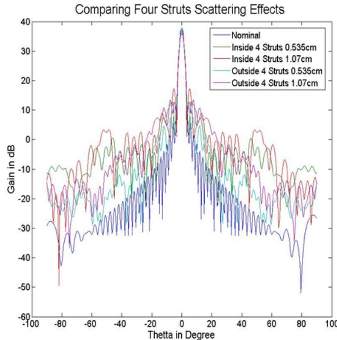
**Fig. 1.7:** Comparing Four Struts Scattering Effects
