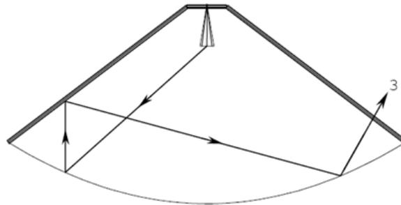
**Fig. 1.2:** Strut scattering of type 3
