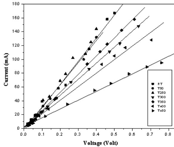
**Fig. 1:** I-V curve for Al-Si sample quenched at different temperatures.
