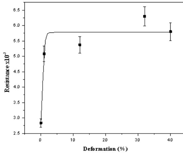
Fig. 4: Electrical resistance as a function of deformation.
