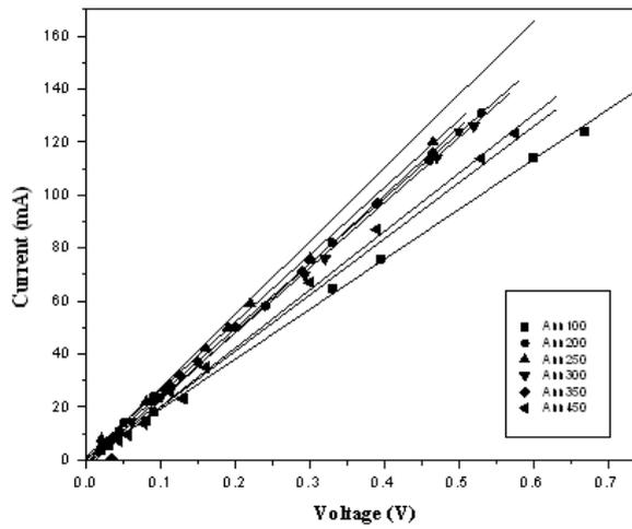
Fig. 5: I-V Curves for Al-Si deformed sample annealed at different temperatures.
