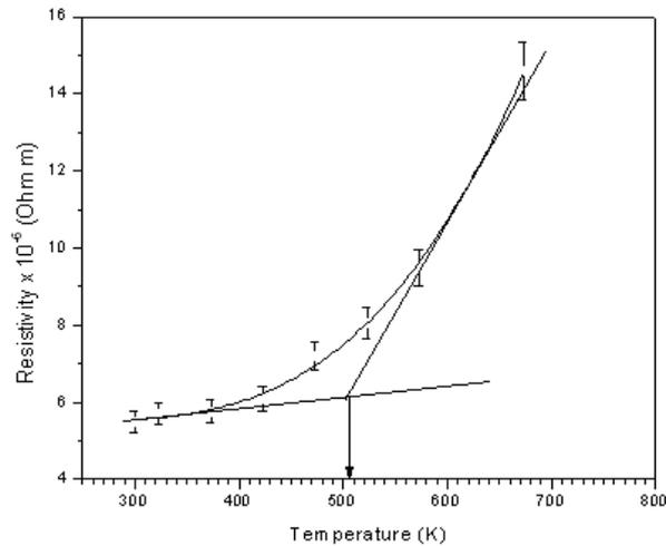
**Fig. 2:** The resistance as a function of quenching temperature.
