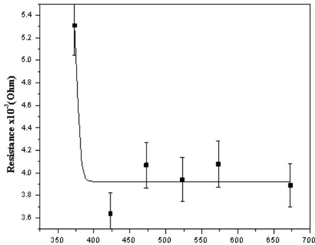
**Fig. 6:** The electrical resistance of the deformed Al-Si sample as a function of annealing temperature.
