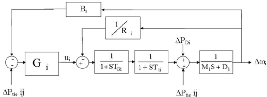
**Fig. 2:** Block diagram for one area of system ( $i^{th}$  area).
