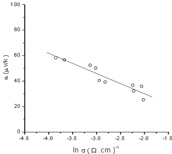
**Fig. 10:** The dependence of the thermoelectric power coefficient on the natural logarithm of the electrical conductivity for TiGaTe<sub>2</sub>
