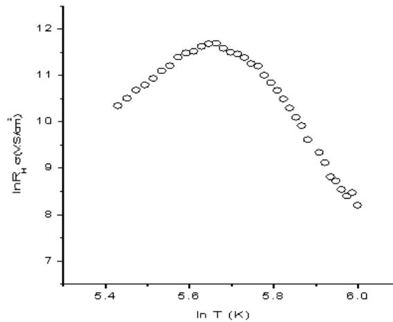
**Fig. 4:** Hall mobility as a function of temperature for TlGaTe<sub>2</sub> single crystal
