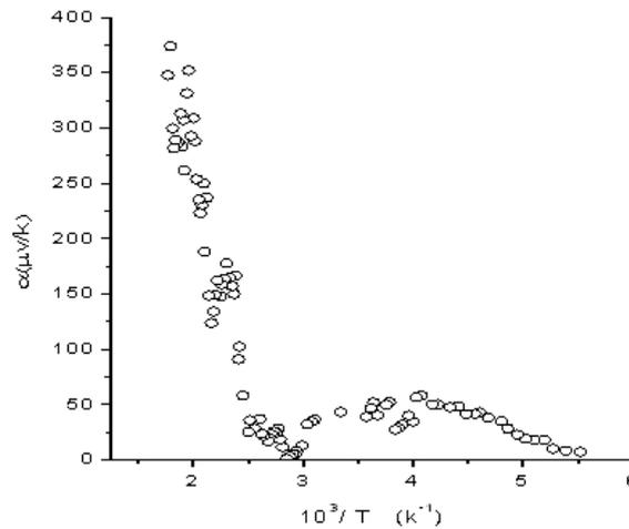
Fig. 7: Plot of  $\alpha$  against  $10^3/T$  for TlGaTe<sub>2</sub> single crystal
