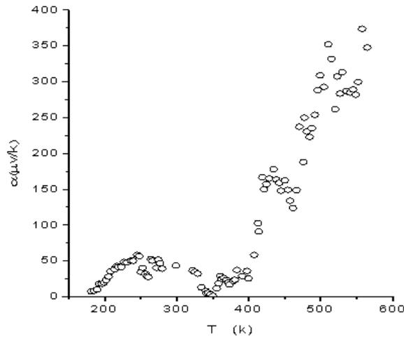
**Fig. 6:** Temperature dependence of TEP for TlGaTe<sub>2</sub> single crystal
