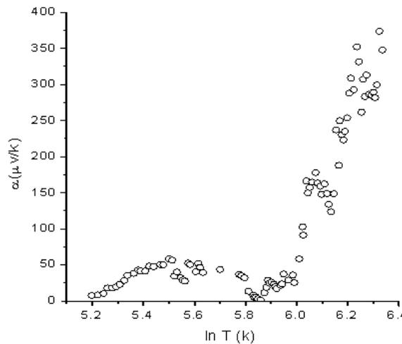
Fig. 8: The relation between  $\alpha$  and  $\ln T$  for for TlGaTe<sub>2</sub> single crystal
