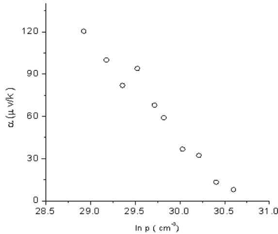
**Fig. 9:** The dependence of the TEP on the natural logarithm of charge carrier concentration for TiGaTe<sub>2</sub> compound
