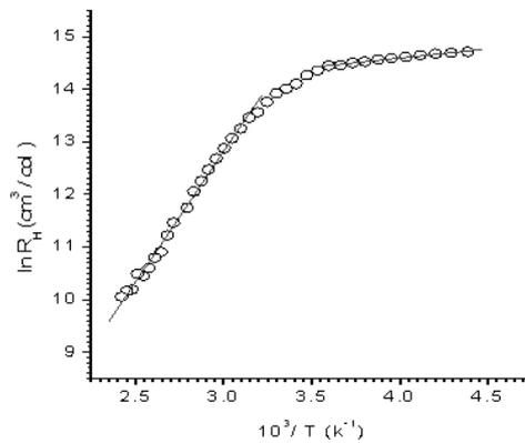
**Fig. 2:** The dependence of  $R_H$  against the temperature for  $\text{TlGaTe}_2$  single crystal
