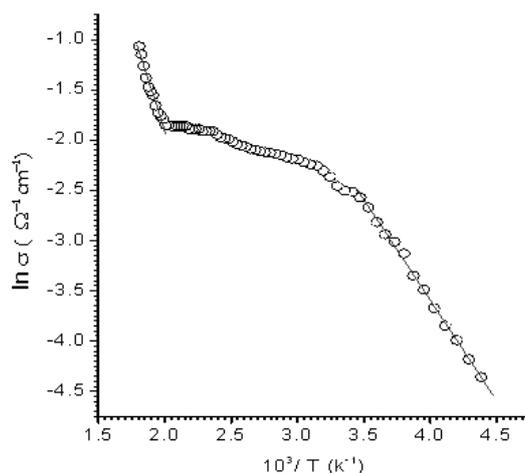
**Fig. 1:** Electrical conductivity of  $\text{TlGaTe}_2$  as a function of temperature
