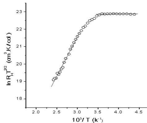
**Fig. 3:** Variation of  $\ln R_H T^{3/2}$  with  $10^3/T$  for  $\text{TlGaTe}_2$  single crystal
