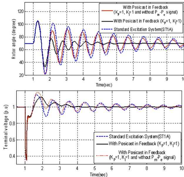
Fig. 7: Rotor angle and terminal voltage of the generator for F1 fault.
