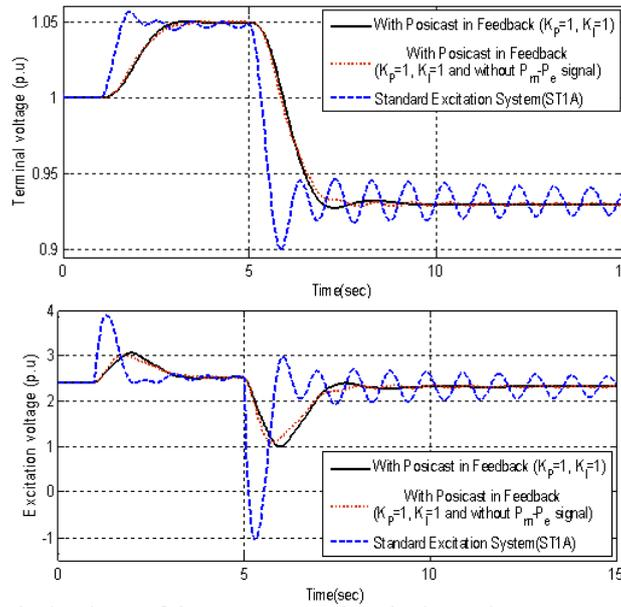
Fig. 6: Terminal voltage of the generator and excitation voltage.
