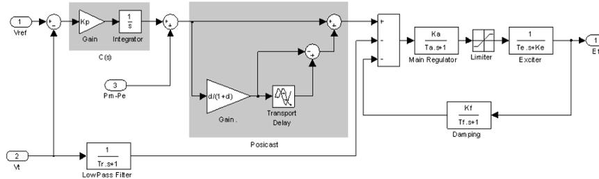
Fig. 5: The AVR and the excitation system after adding POSICAST.
