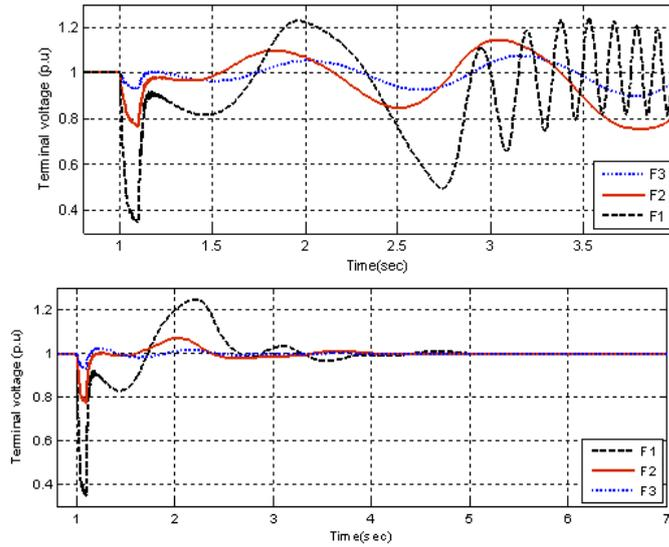
**Fig. 10:** Terminal voltage of the generator with standard excitation system (upper) and with using the POSICAST in feedback (lower) ( $K_p=1, K_i=1$  and with  $P_m-P_e$  signal).
