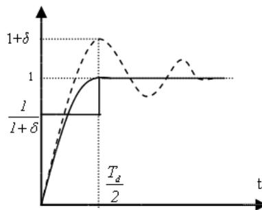
**Fig. 1:** Step Response of the system with (solid line) and without (dashed line) POSICAST and the control signal generated by POSICAST
