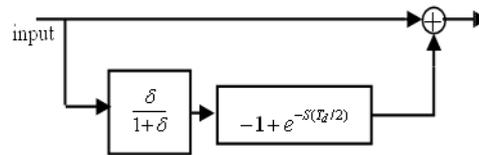
**Fig. 2:** Open-loop half cycle POSICAST.
