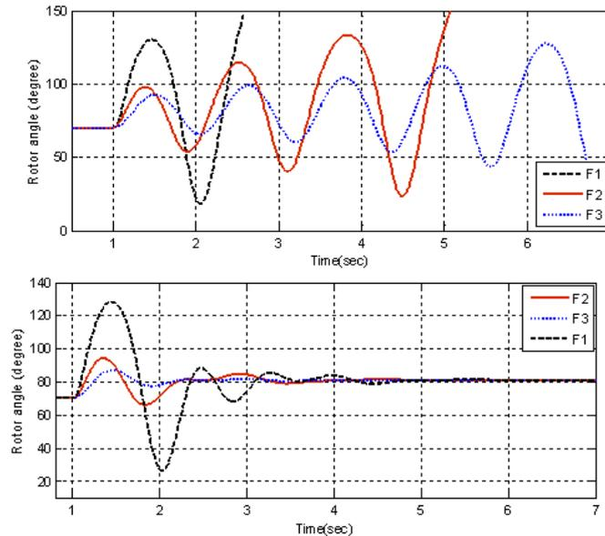
**Fig. 9:** Rotor angle with standard excitation system (upper) and with using the POSICAST in feedback (lower) ( $K_p=1, K_i=1$  and with  $P_m-P_e$  signal).
