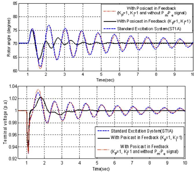
**Fig. 8:** Rotor angle and terminal voltage of the generator for F3 fault.
