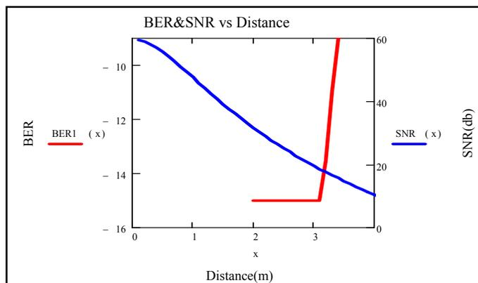
Fig. 3: SNR (db) & BER versus Distance (m).
