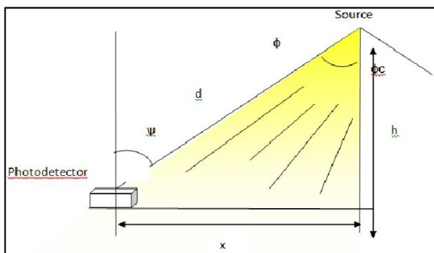
**Fig. 1:** The propagation model of direct links.
