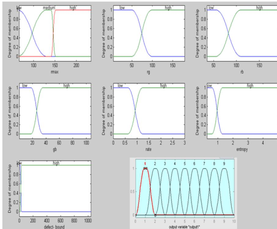
Fig. 2: Membership Functions For Input, Output.
