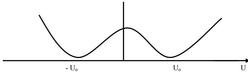
**Fig. 2:** A double – well potential form used in  $\phi^4$  and SSH models.
