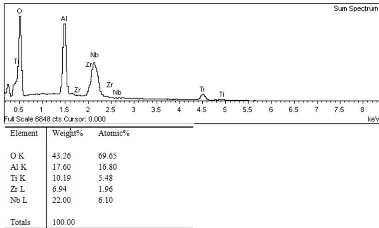
**Fig. 3:** EDX map and composition percentages analysis of sand blasted and sulfuric acid etched Ti13Zr13Nb.
