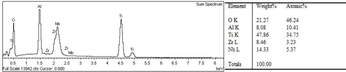
**Fig. 2:** EDX map and composition percentages analysis of sand blasted Ti13Zr13Nb.
