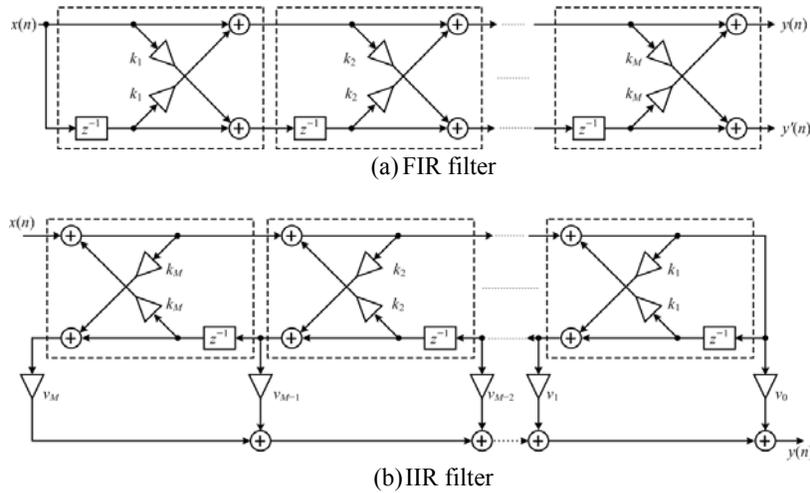
**Fig. 8:** Lattice form realization of  $M$ -th (a) FIR lattice filter and (b) IIR lattice filter.
