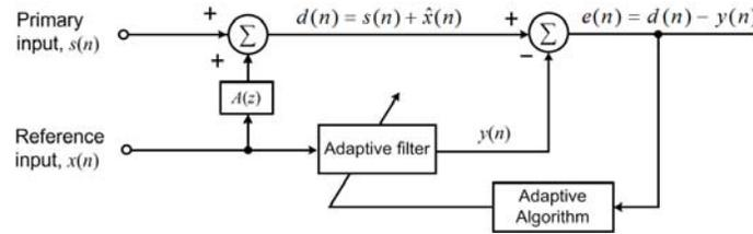
**Fig. 1:** Block diagram of adaptive noise cancellation system
