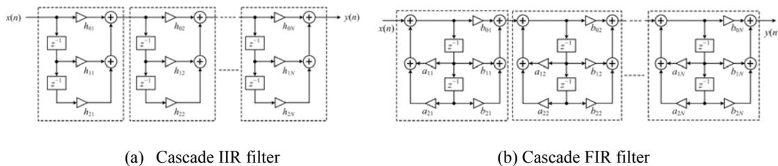
**Fig. 5:** The second-order filter sections of (a) cascade FIR filter and (b) cascade IIR filter.
