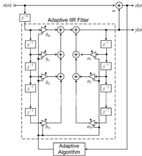
**Fig. 4:** Structure of ALE with direct-form adaptive IIR filter.
