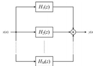
**Fig. 6:** The parallel structure of  $H(z)$ .
