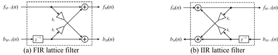
**Fig. 7:** Basic block of two-multiplier and a delay of (a) FIR lattice filter and (b) IIR lattice filter.
