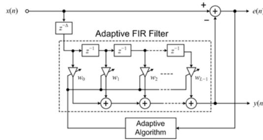
**Fig. 3:** Block diagram of FIR-ALE filter.
