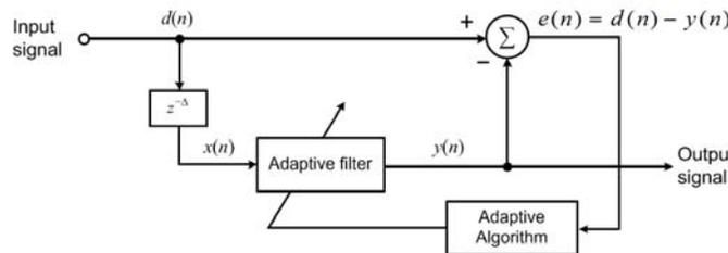
**Fig. 2:** Block diagram of adaptive line enhancer
