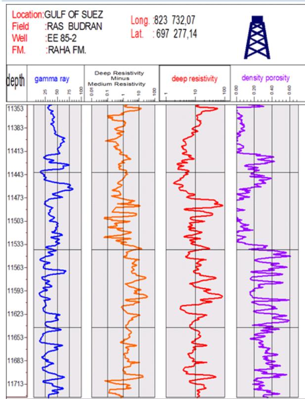
Fig. 9: Discrimination of effective from ineffective porosity in EE85-2 well.
