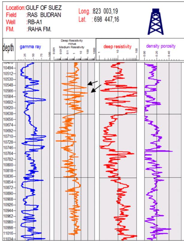
Fig. 2: Discrimination of effective from ineffective porosity in RB-A1 well.
