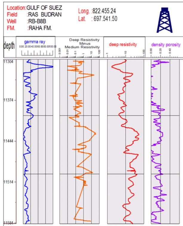
Fig. 6: Discrimination of effective from ineffective porosity in RB-B8B well.
