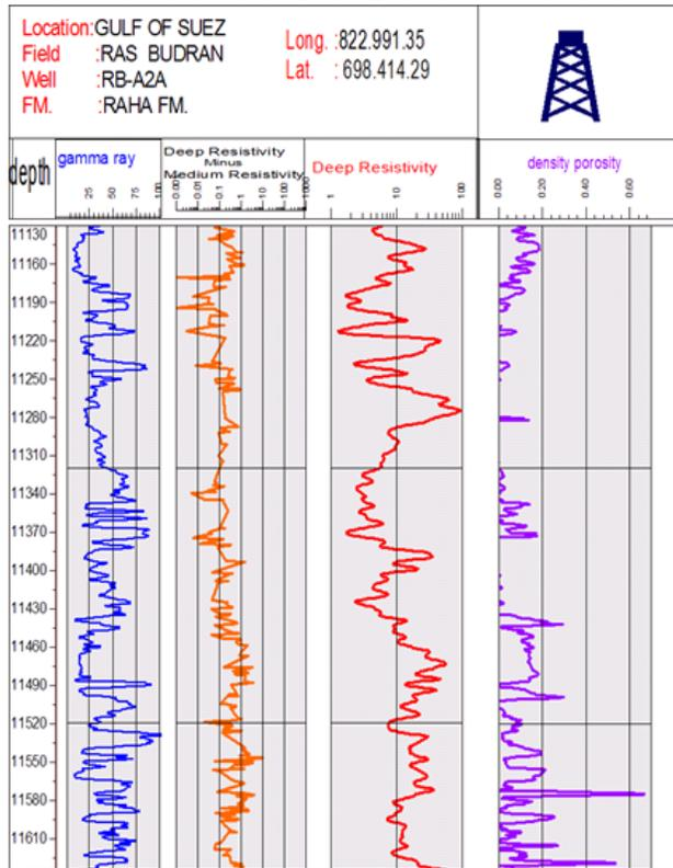
Fig. 3: Discrimination of effective from ineffective porosity in RB-A2A well.
