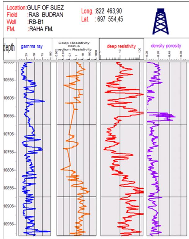
**Fig. 4:** Discrimination of effective from ineffective porosity in RB-B1 well.
