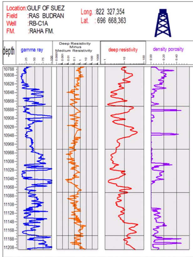
Fig. 7: Discrimination of effective from ineffective porosity in RB-C1A well.
