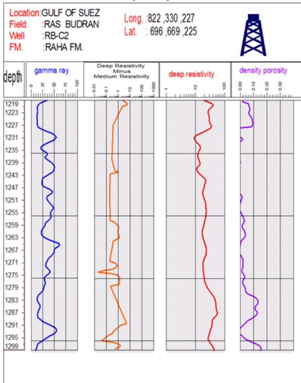
Fig. 8: Discrimination of effective from ineffective porosity in RB-C2 well.
