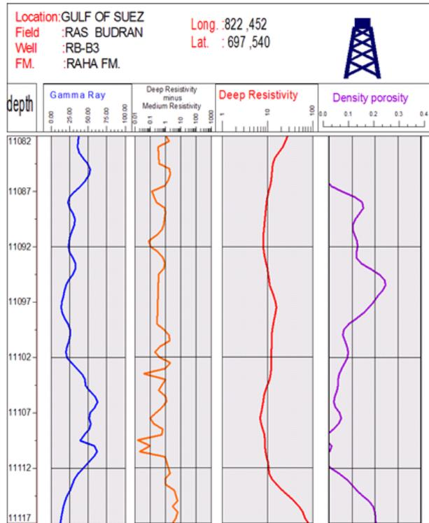
Fig. 5: Discrimination of effective from ineffective porosity in RB-B3 well.
