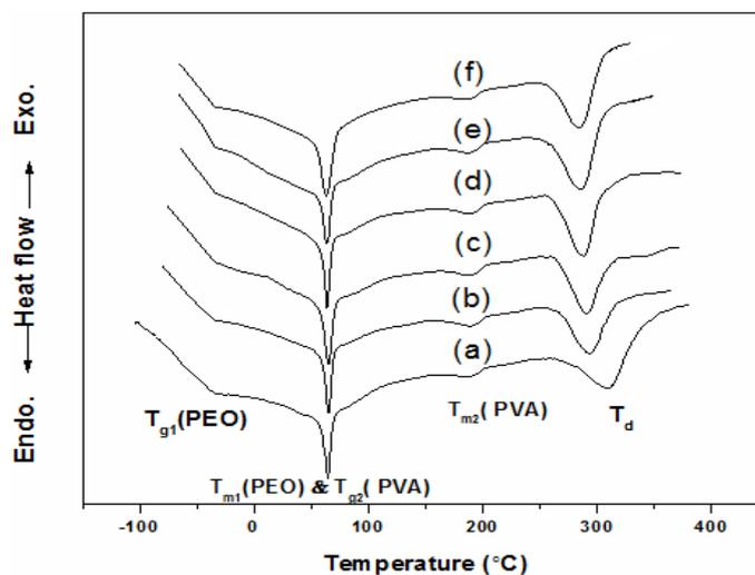
**Fig. 10:** DSC of: (a) 50/50 (wt/wt. %) PEO/PVA undoped blend sample and blend sample doped with: (b) 0.5, (c) 1.0, (d) 2.5, (e) 5 and (f) 10 wt. % ZnO nanoparticles.
