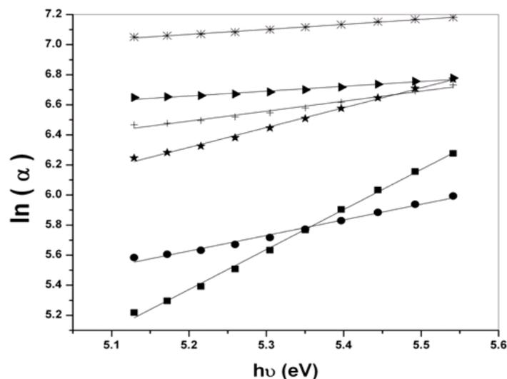
**Fig. 8:** Relation between  $\ln(\alpha)$  versus  $h\nu$  for (■) 50/50 (wt/wt. %) PEO/PVA undoped blend sample and blend sample doped with; (●) 0.5, (★) 1.0, (+) 2.5, (▶) 5.0 and (\*) 10.0 wt% ZnO nanoparticles.
