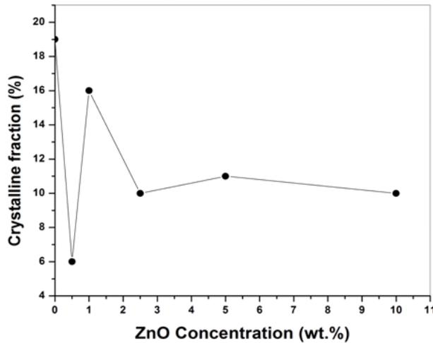
**Fig. 3:** Variation in crystalline fraction for 50/50 (wt/wt. %) PEO/PVA as a function of ZnO concentration.
