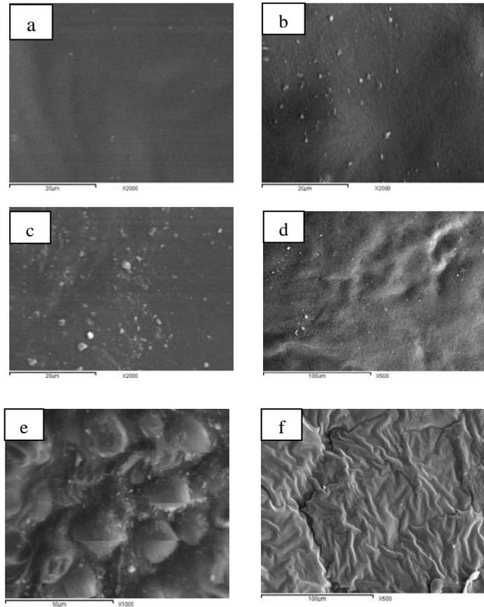
**Fig. 9:** SEM images of: (a) 50/50 (wt/wt. %) PEO/PVA undoped blend sample and blend sample doped with: (b) 0.5, (c) 1.0, (d) 2.5, (e) 5 and (f) 10 wt. of % ZnO nanoparticles.
