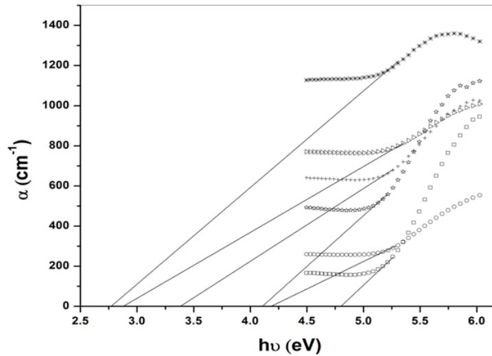
**Fig. 7:** Relation between absorbance coefficient ( $\alpha$ ) versus  $h\nu$  for ( $\square$ ) 50/50 (wt/wt. %) PEO/PVA undoped blend sample and blend sample doped with; ( $\circ$ ) 0.5, ( $\star$ ) 1.0, ( $+$ ) 2.5, ( $\triangle$ ) 5.0 and ( $*$ ) 10.0 wt% ZnO nanoparticles.
