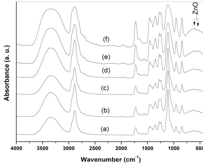
**Fig. 5:** FT-IR absorption spectra of: (a) (50/50wt/wt. %) PEO/PVA undoped blend sample and blend sample doped with: (b) 0.5, (c) 1.0, (d) 2.5, (e) 5.0 and (f) 10wt% of ZnO nanoparticles.
