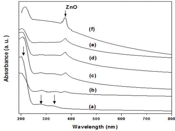
**Fig. 6:** UV-vis spectra of: (a) 50/50 (wt/wt. %) PEO/PVA undoped blend sample and blend sample doped with: (b) 0.5, (c) 1.0, (d) 2.5, (e) 5.0 and (f) 10 wt. % ZnO nanoparticles.
