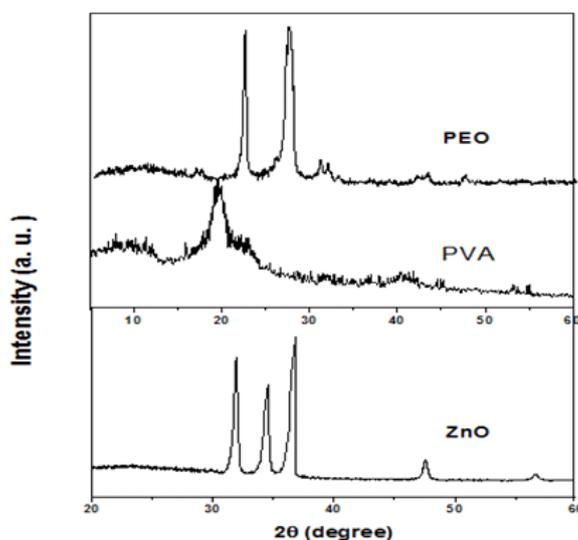
**Fig. 1:** X-ray diffraction of ZnO, PVA and PEO.
