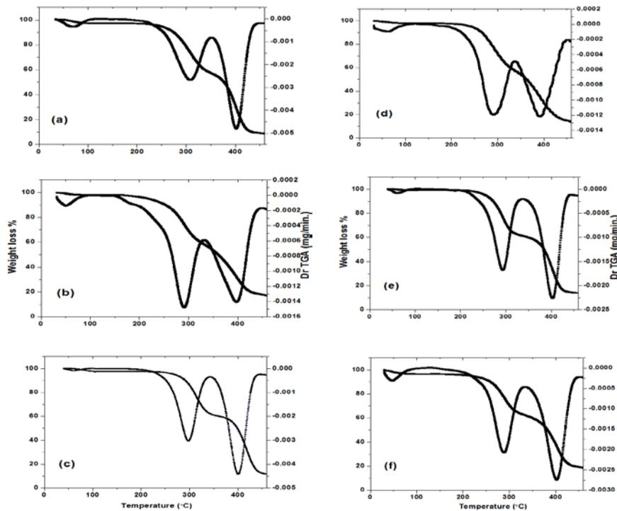
**Fig. 11:** TGA& Dr TGA of: (a) 50/50 (wt/wt. %) PEO/PVA undoped blend sample and blend sample doped with: (b) 0.5, (c) 1.0, (d) 2.5, (e) 5.0 and (f) 10 wt. % ZnO nanoparticles.
