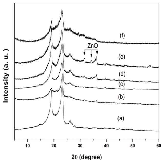
**Fig. 2:** X-ray diffraction of: (a) 50/50 (wt/wt. %) PEO/PVA undoped blend sample and blend sample doped with: (b) 0.5, (c) 1.0, (d) 2.5, (e) 5.0 and (f) 10 wt. % ZnO nanoparticles
