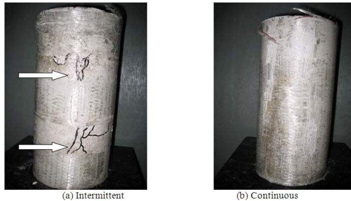
Fig. 7: Cylindrical Specimens Strengthened with GFRP Materials.
