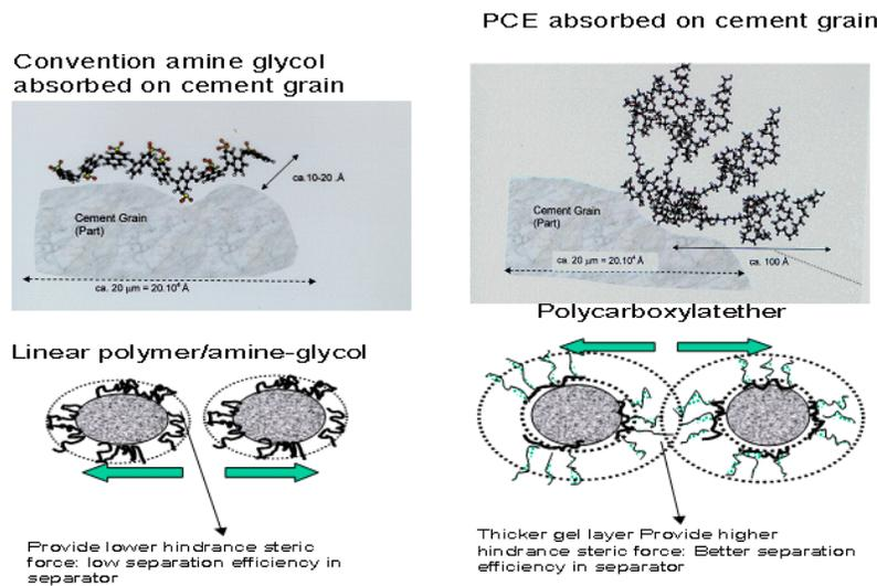
**Fig. 2:** Hindrance steric force dispersion for PCE when absorbed on cement grain.
