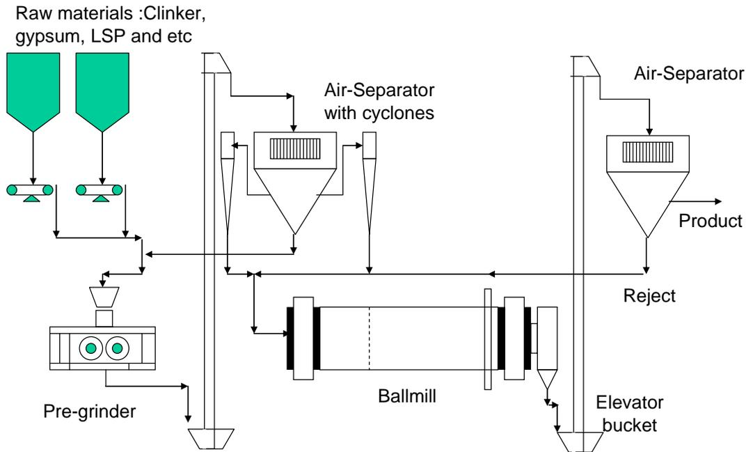
**Fig. 1:** Simplified configuration process for a closed circuit system of the studied cement plant.
