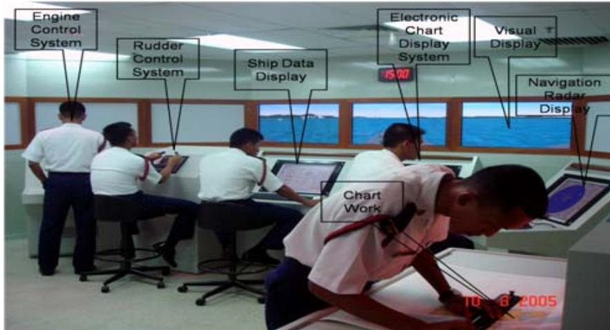
**Fig. 2:** The picture of Ship Navigation Simulator at NDUM (MOHE, 2011).
