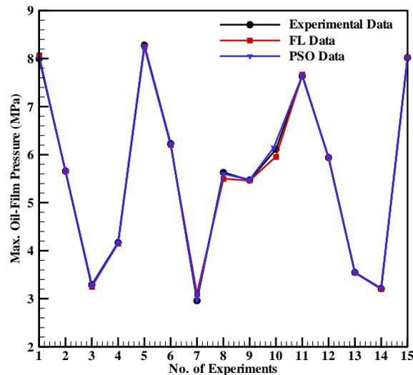
**Fig. 12:** Experimental data vs. predicted data by FL and PSO
