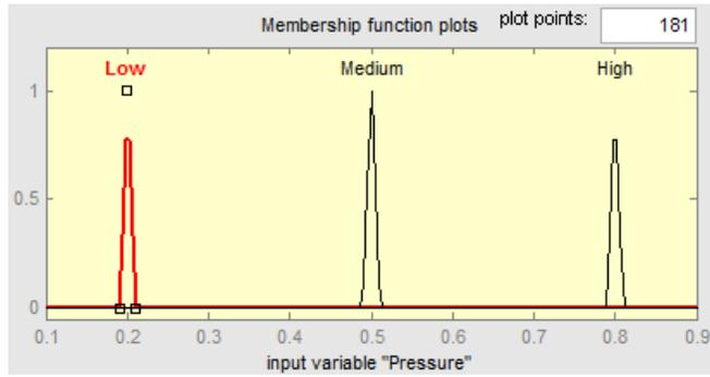
Fig. 7: Oil-feed pressure input membership function
