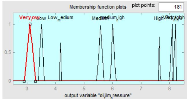
Fig. 8: Oil-film pressure output membership function
