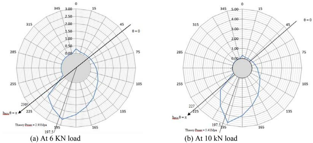
**Fig. 4:** Experimental pressure distribution around the journal bearing circumference
