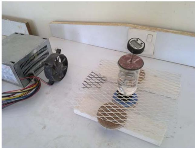
**Fig. 3:** method of measuring water temperature gain and ignition period of the briquettes
