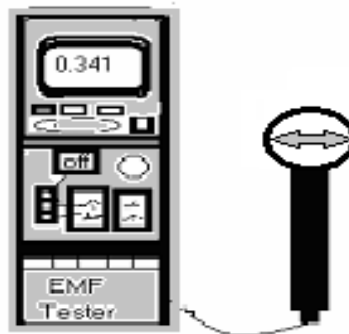
Fig. 1: The electromagnetic field tester: (EMF-827) with wireless probe.
